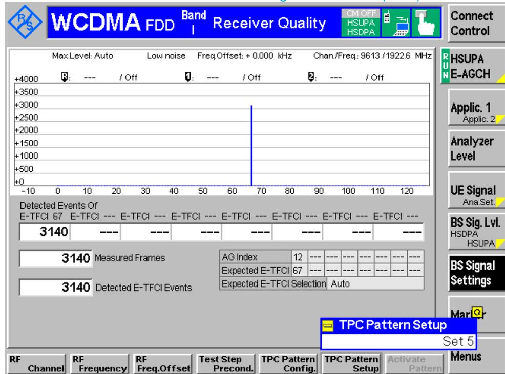
Figure 8(a): Target E-TFCI transmitted by the UE for Subtest 5
