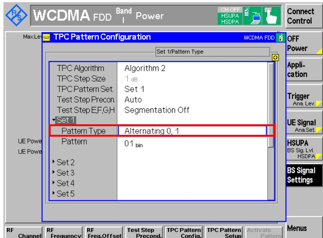
Figure 10: Alternating “0” and “1” TPC pattern configuration
