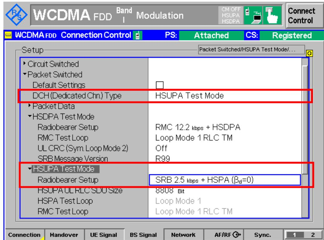
**Figure 1(c): SRB 2.5 kbps + HSPA 34.108 configuration**
