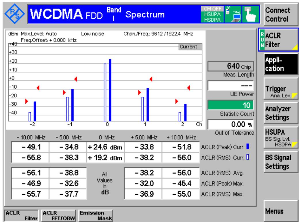
Figure 14: ACLR with E-DCH measurement result
