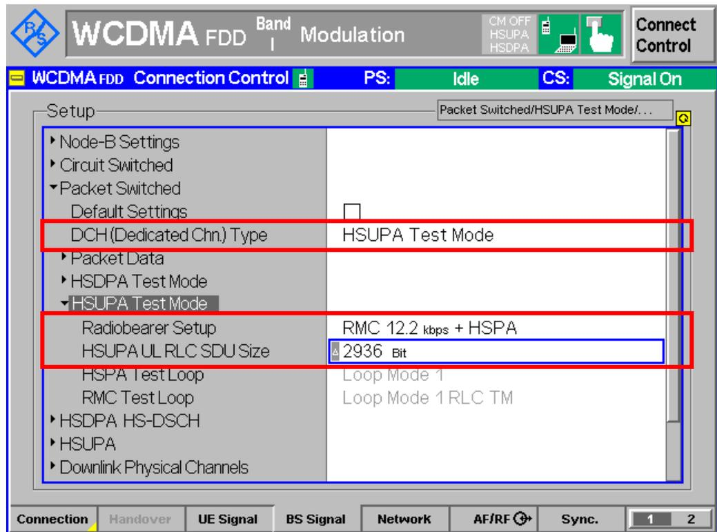
Figure 1(b): RMC 12.2 kbps + HSPA 34.108 configuration
