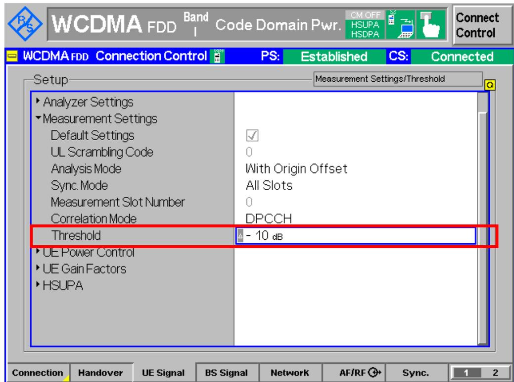
Figure 16: Measurement threshold configuration
