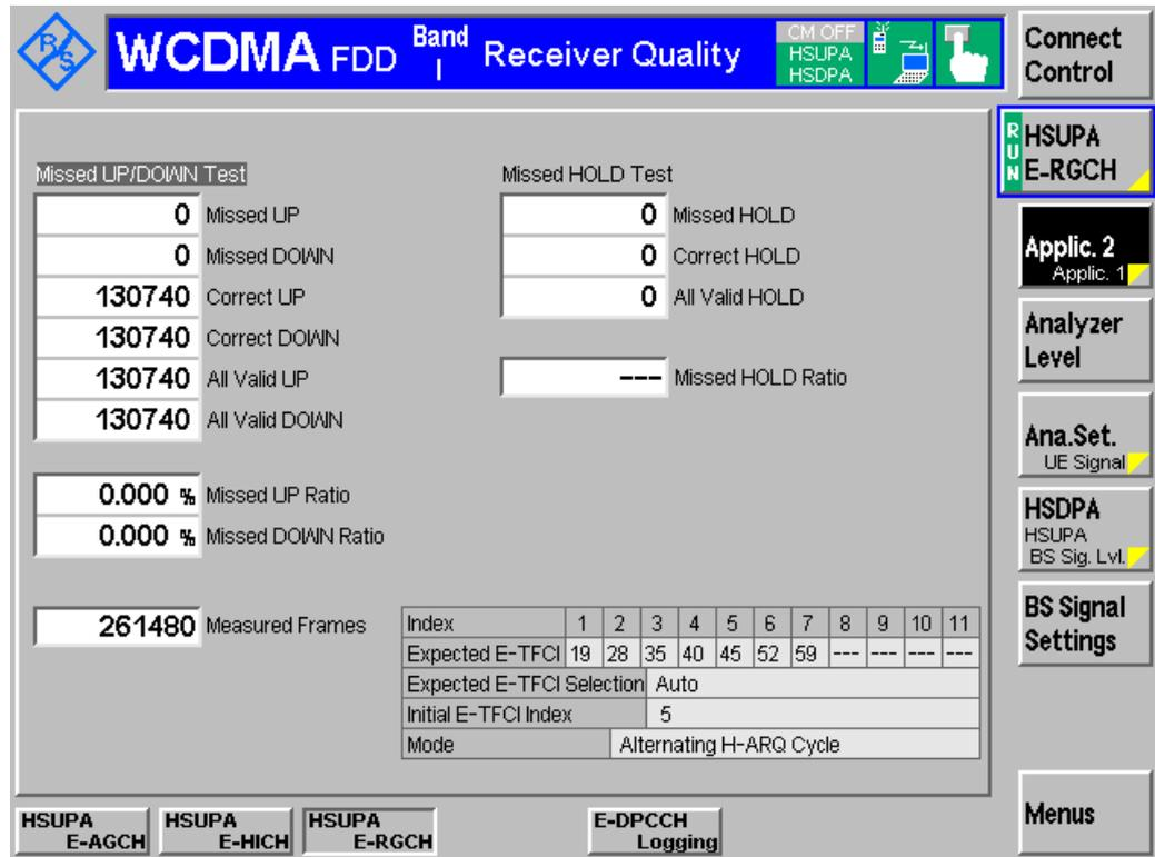
Figure 21(a): E-RGCH Missed UP/DOWN measurement result
