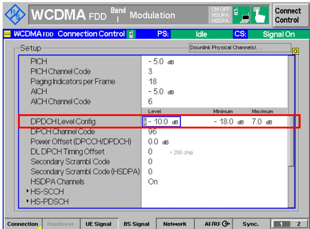
Figure 5(c): Downlink physical channels configuration according to Table 9
