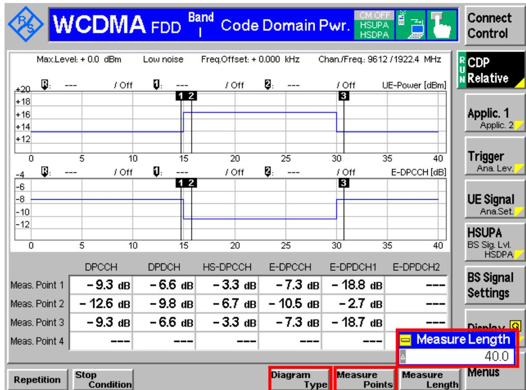
Figure 12(b): CDP Relative diagram configuration
