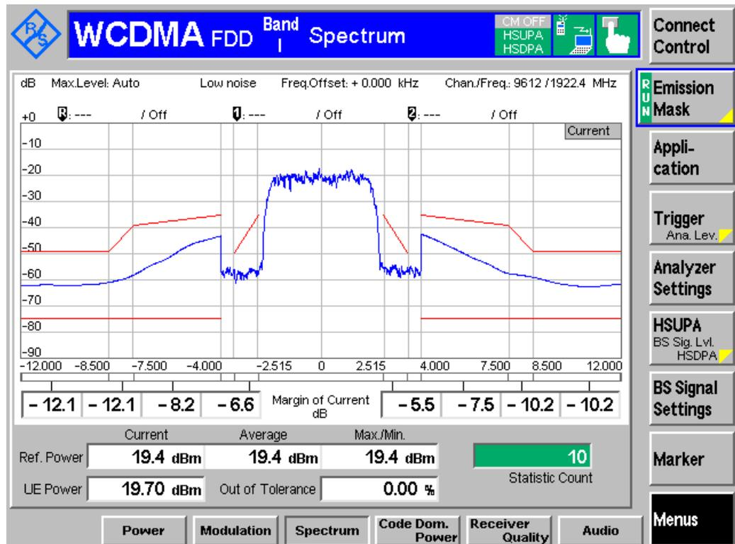
Figure 13: Spectrum emission mask measurement result
