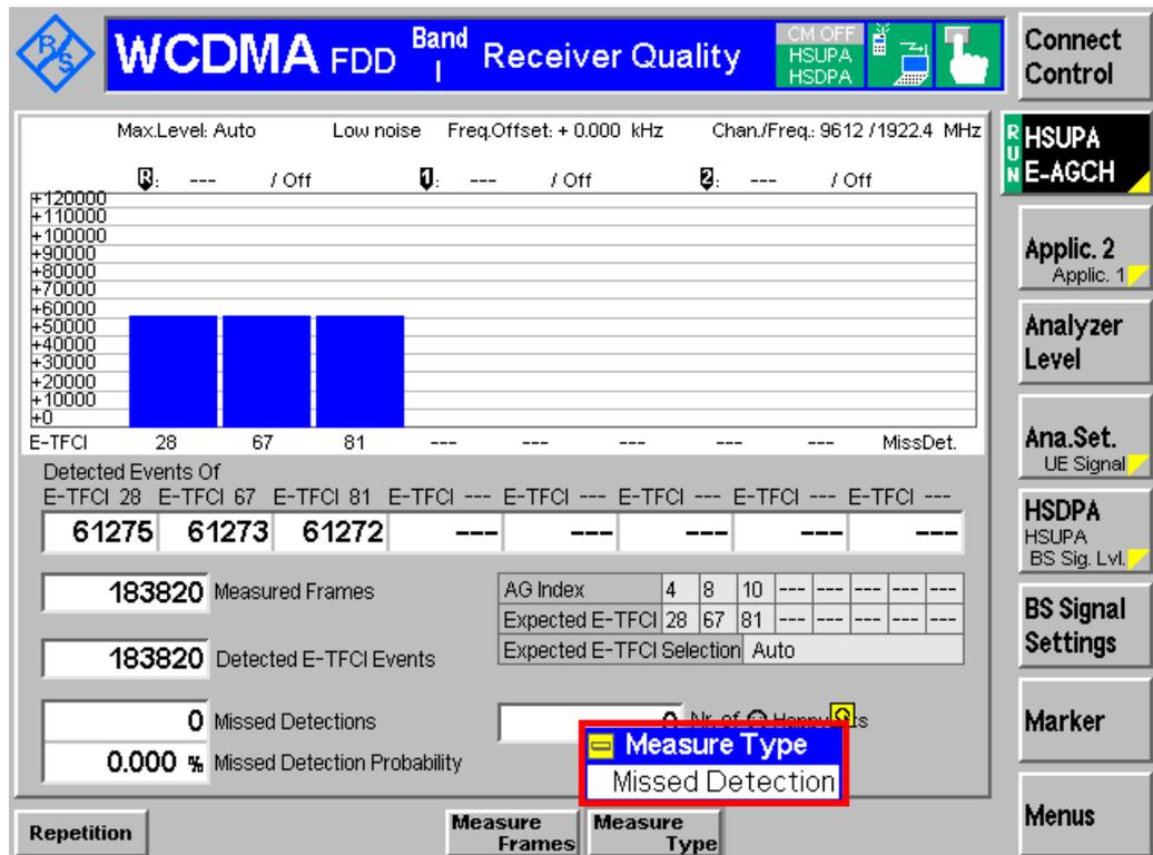
**Figure 22: E-AGCH missed detection measurement result**
