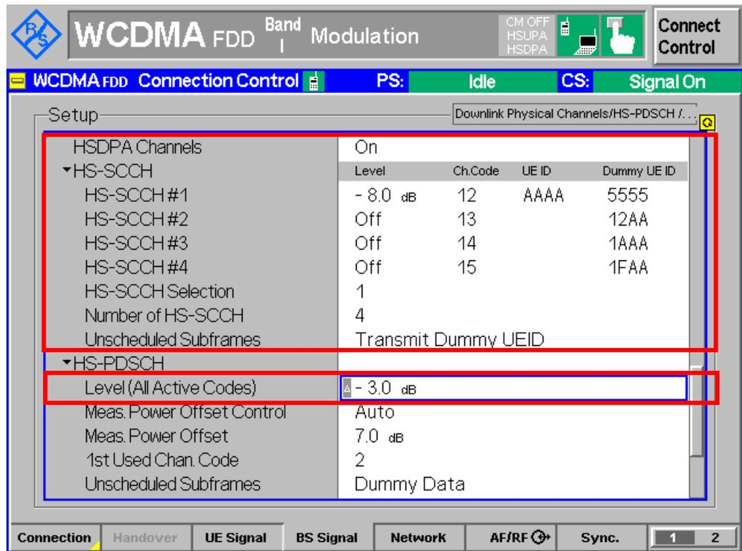
Figure 5(d): Downlink physical channels configuration according to Table 9
