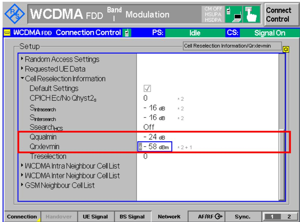
Figure 4(a) : Setting for the serving cell
