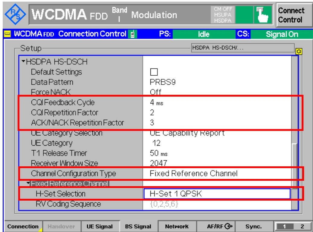
Figure 2(a): RADIO BEARER SETUP message configuration
