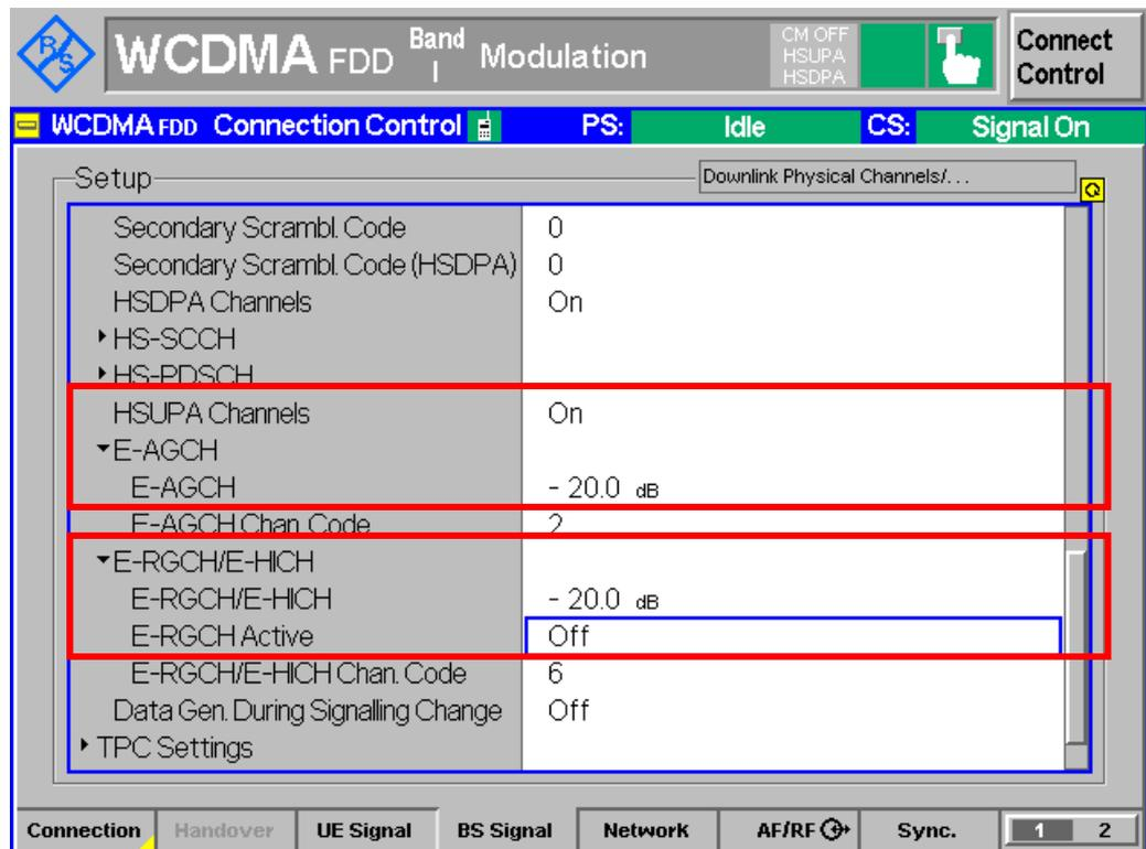
Figure 5(e): Downlink physical channels configuration according to Table 9
