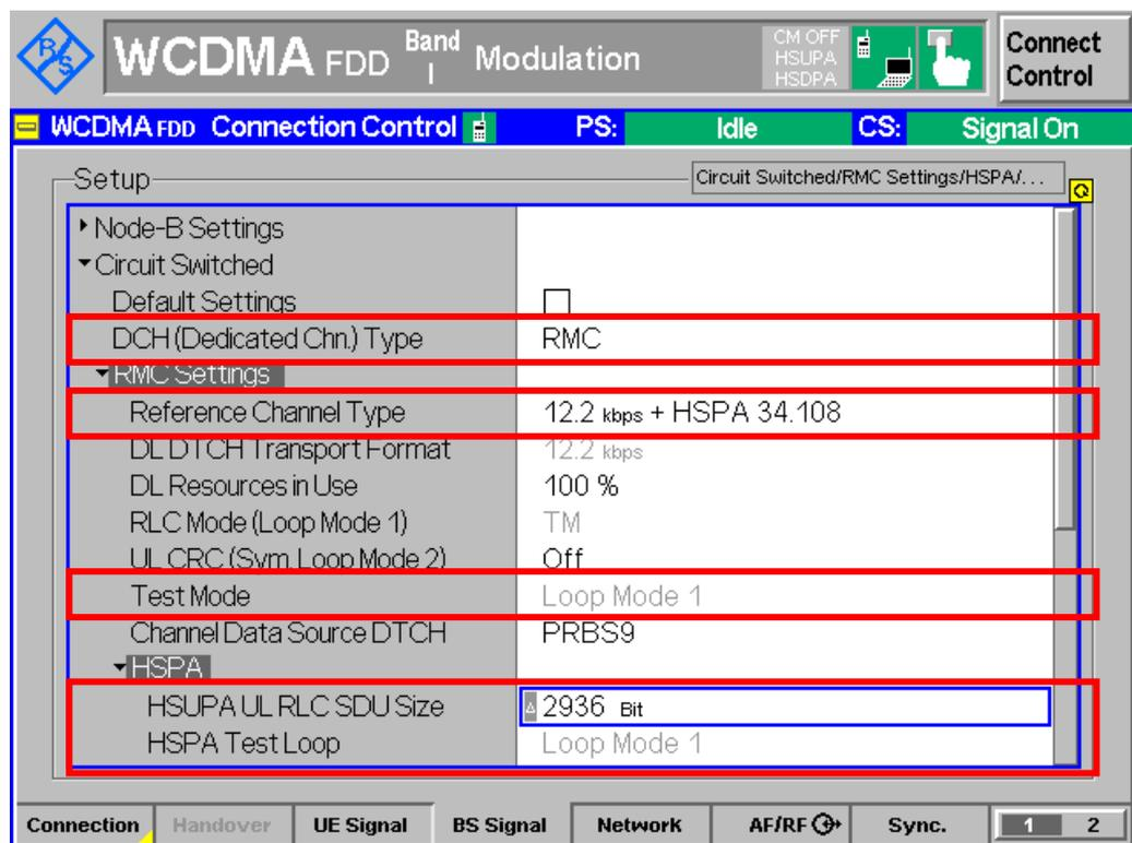
Figure 1(a): RMC 12.2 kbps + HSPA 34.108 configuration
