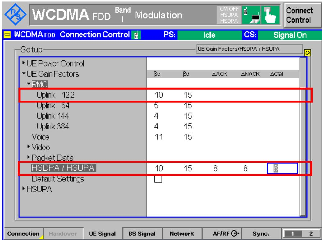
Figure 3(a):  $\beta$  values for transmitter characteristics tests with HS-DPCCH and E-DCH configuration
