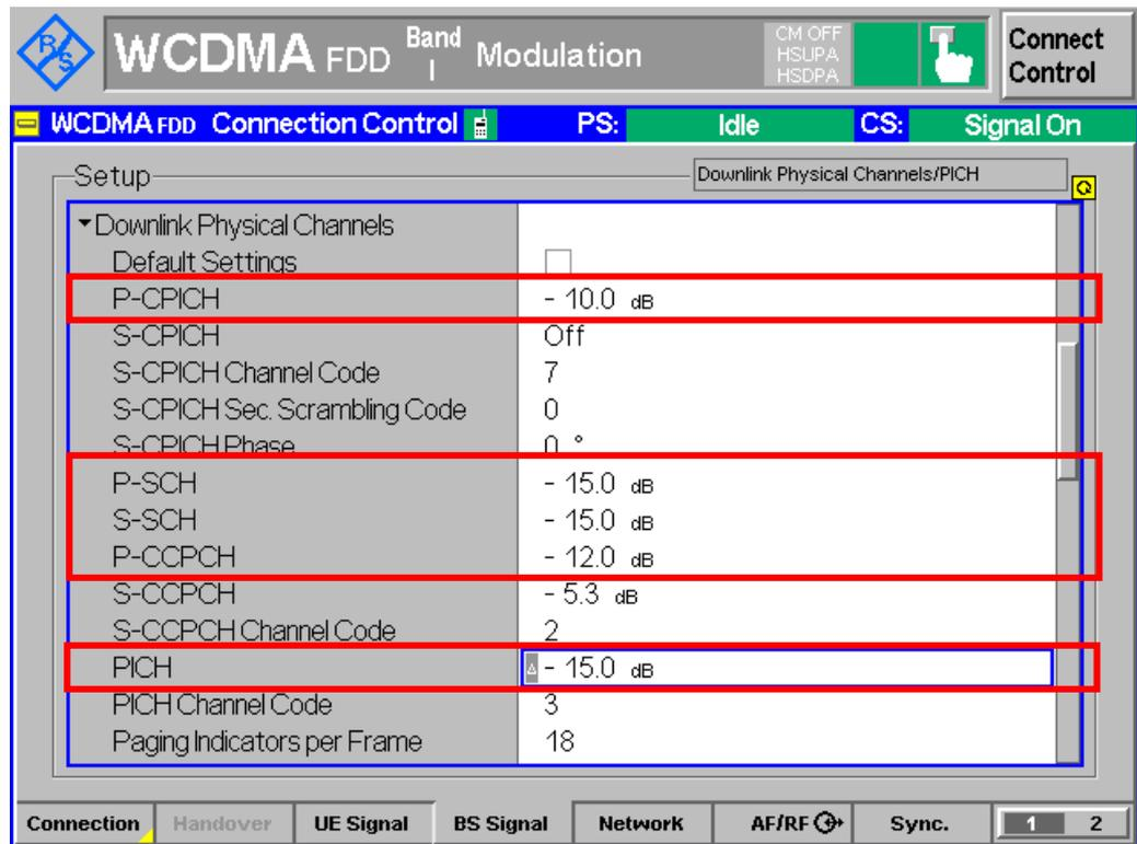
Figure 5(b): Downlink physical channels configuration according to Table 9
