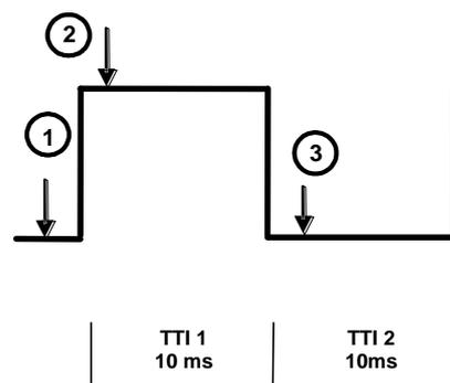
Figure 9: Transmit power profile showing measurement points (Figure 5.2D.1 of TS 34.121 [1])
