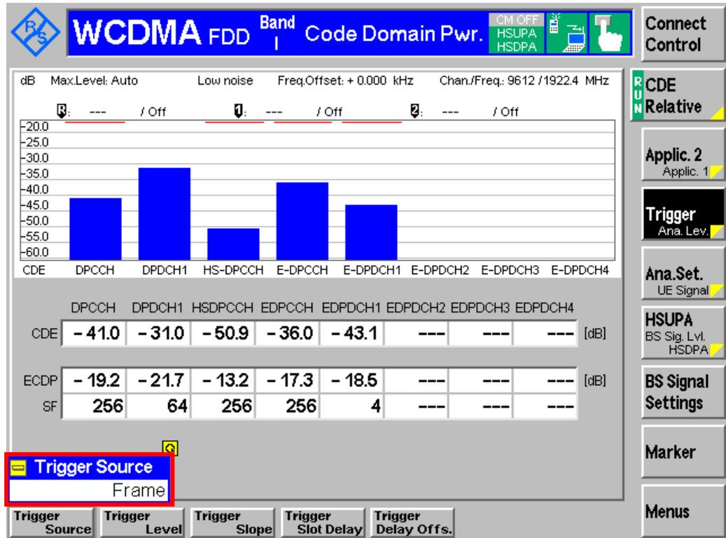
Figure 15: Relative code domain error with HS-DPCCH and E-DCH measurement result
