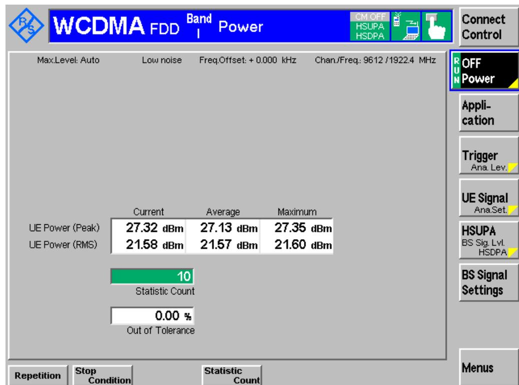
Figure 8: Maximum output power with HS-DPCCH and E-DCH measurement result
