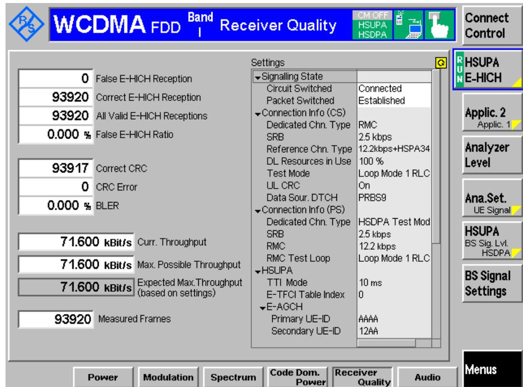
Figure 18: Detection of E-DCH HARQ Indicator Channel (E-HICH) measurement result
