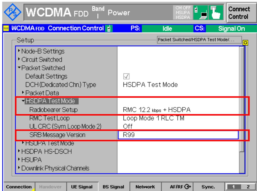
Figure 1(b): HSDPA Test Mode configuration
