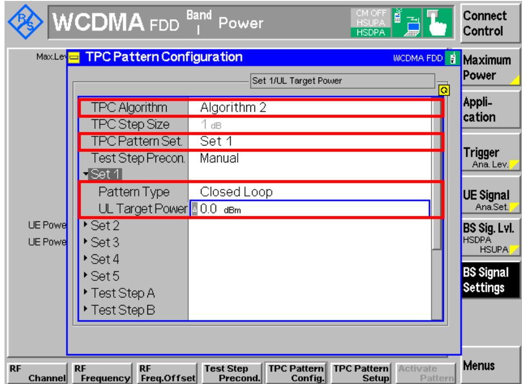
Figure 12(a): Algorithm 2 TPC pattern configuration
