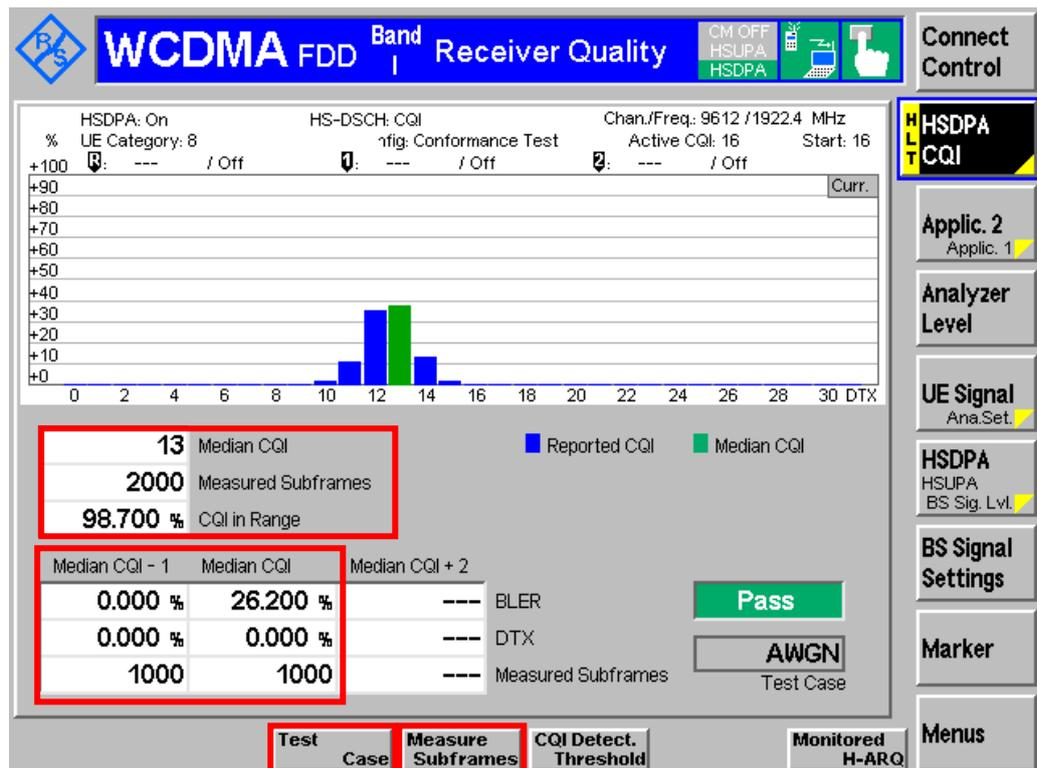
Figure 30: HSDPA CQI (AWGN propagation conditions) measurement result
