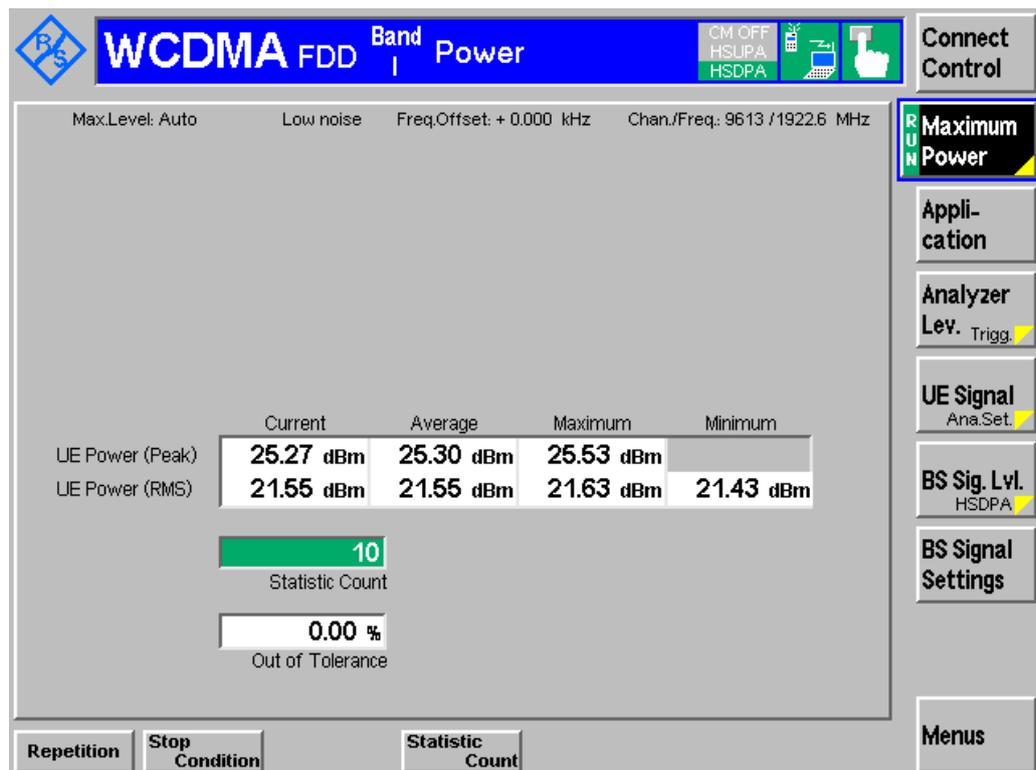
Figure 9: Maximum output power with HS-DPCCH measurement result
