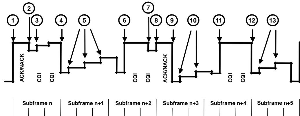
Figure 17: Transmit power template at max power with TPC\_cmd = 1 (Figure 5.7A.3 of TS 34.121 [1])
