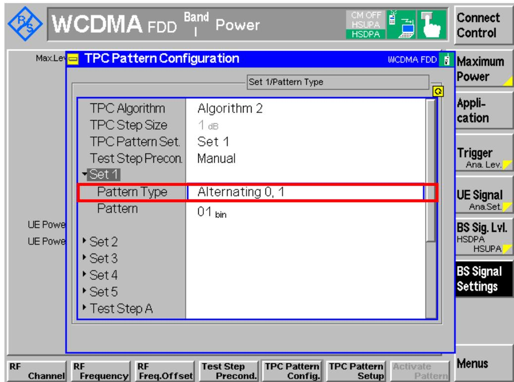
Figure 12(b): Algorithm 2 TPC pattern configuration
