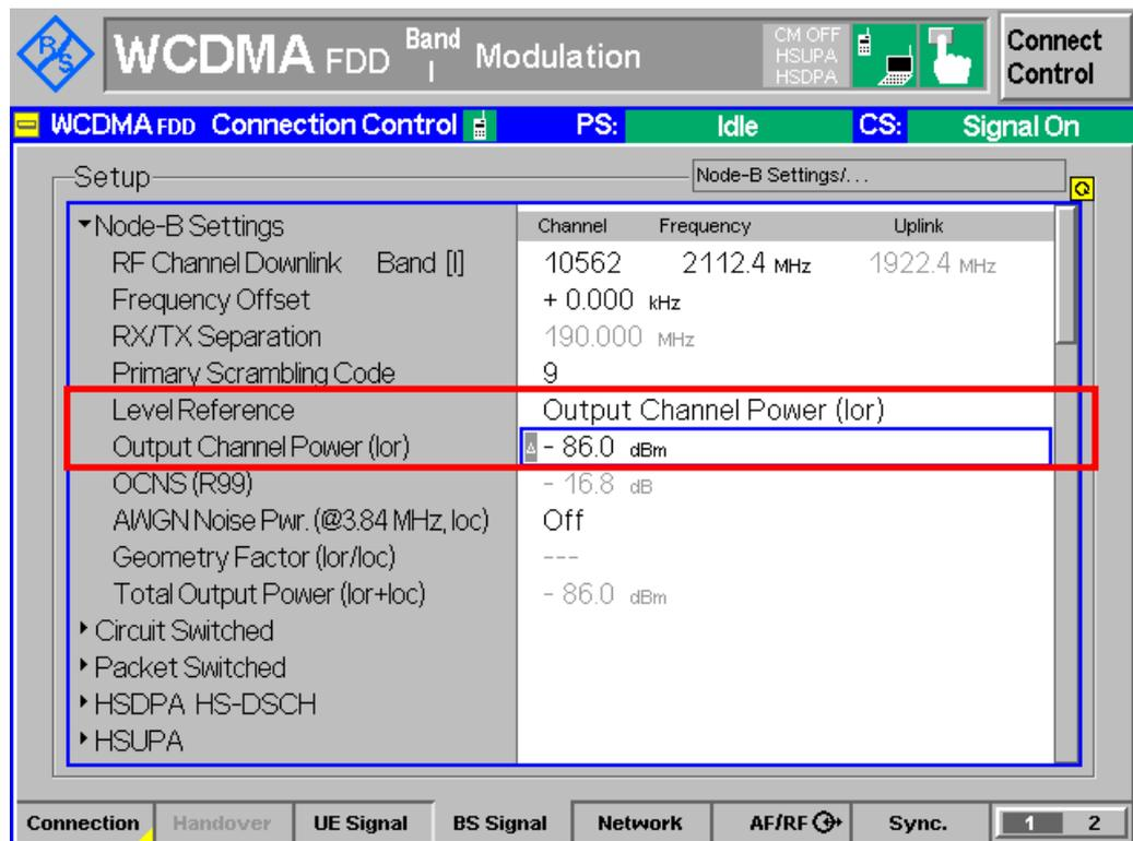
Figure 6(a) : Downlink physical channels configuration according to Table 5(a) and Table 5(b)
