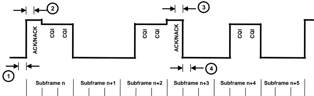
**Figure 22: HS-DPCCH on/off pattern showing measurement positions (Figure 5.13.1A.1 and Figure 5.13.1AA.1 of TS 34.121 [1])**
