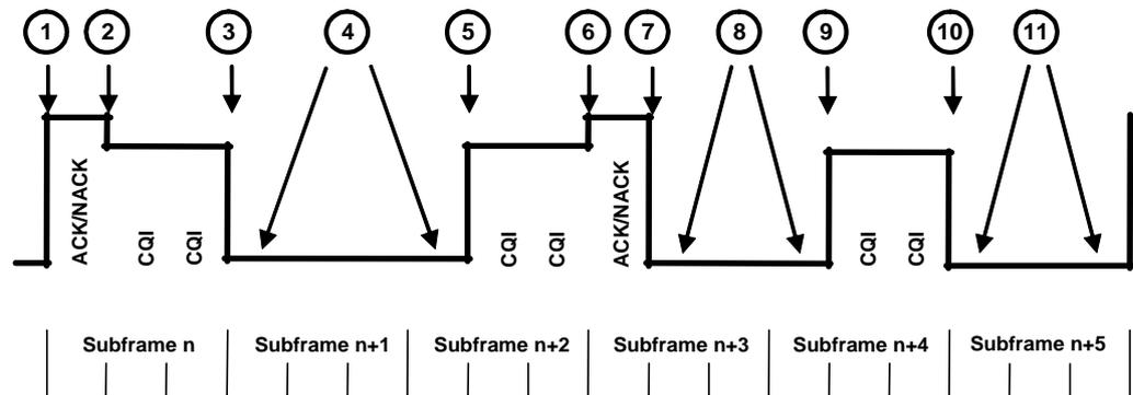
Figure 16: Transmit power template below max power with  $TPC\_cmd = 0$  (Figure 5.7A.2 of TS 34.121 [1])
