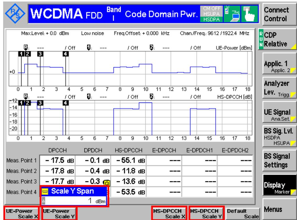
Figure 14(b): Span of X and Y scale configuration
