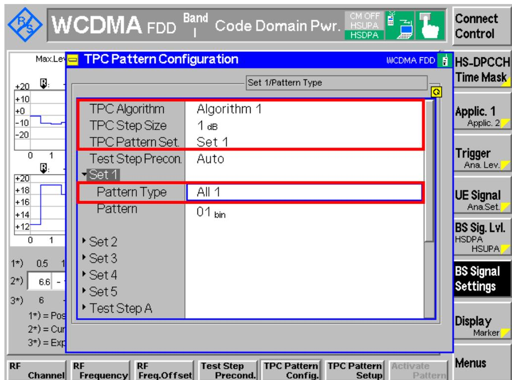
Figure 18: Algorithm 1 TPC pattern configuration
