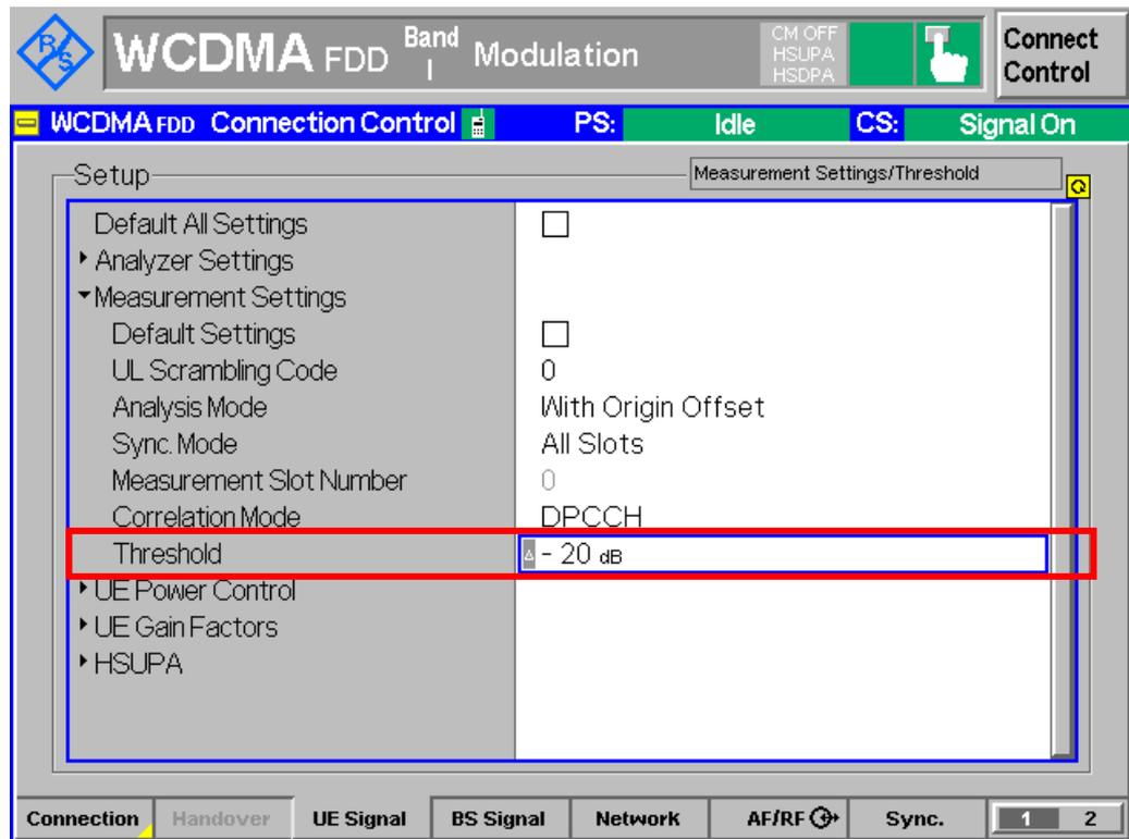
Figure 13: Measurement threshold configuration
