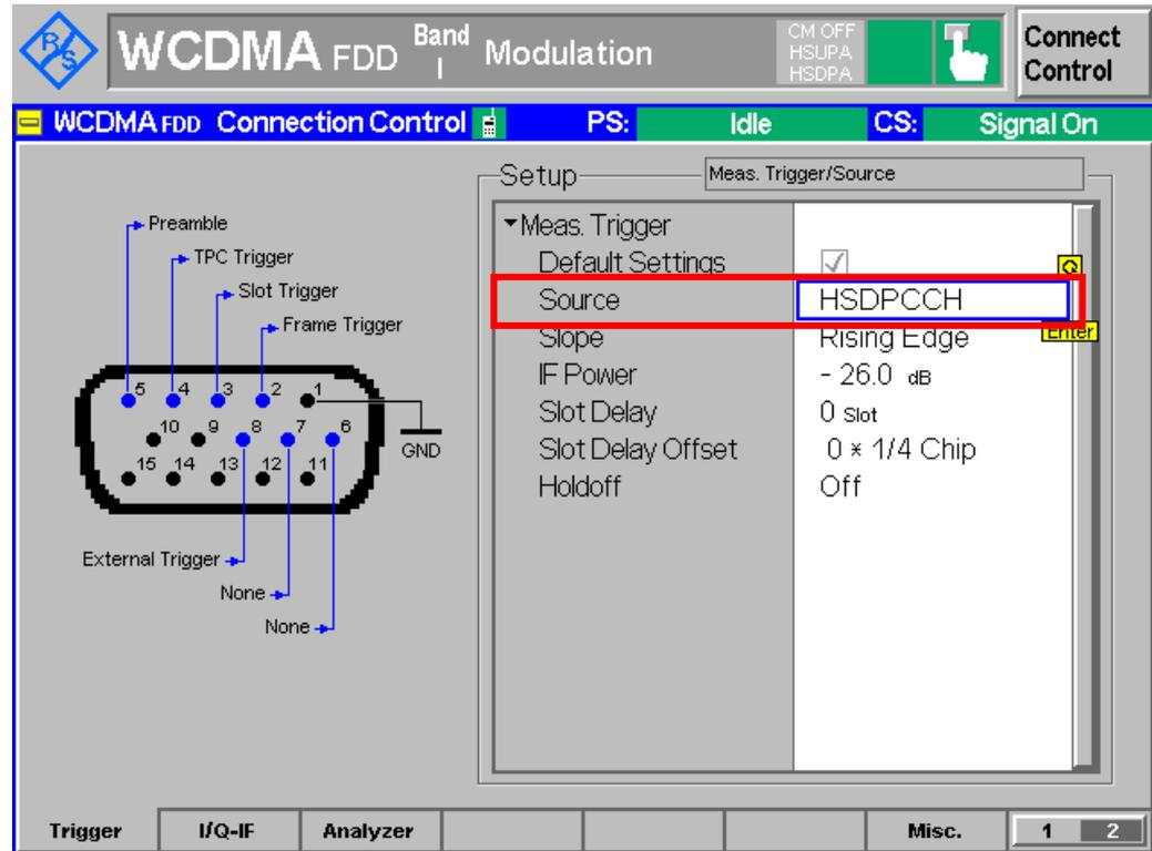
Figure 8: HS-DPCCH trigger configuration
