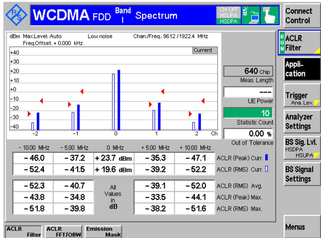
Figure 21: ACLR with HS-DPCCH measurement result
