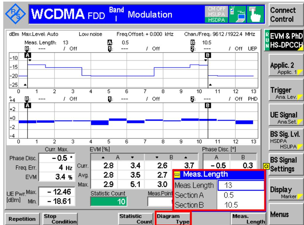
Figure 25: EVM and phase discontinuity with HS-DPCCH measurement result
