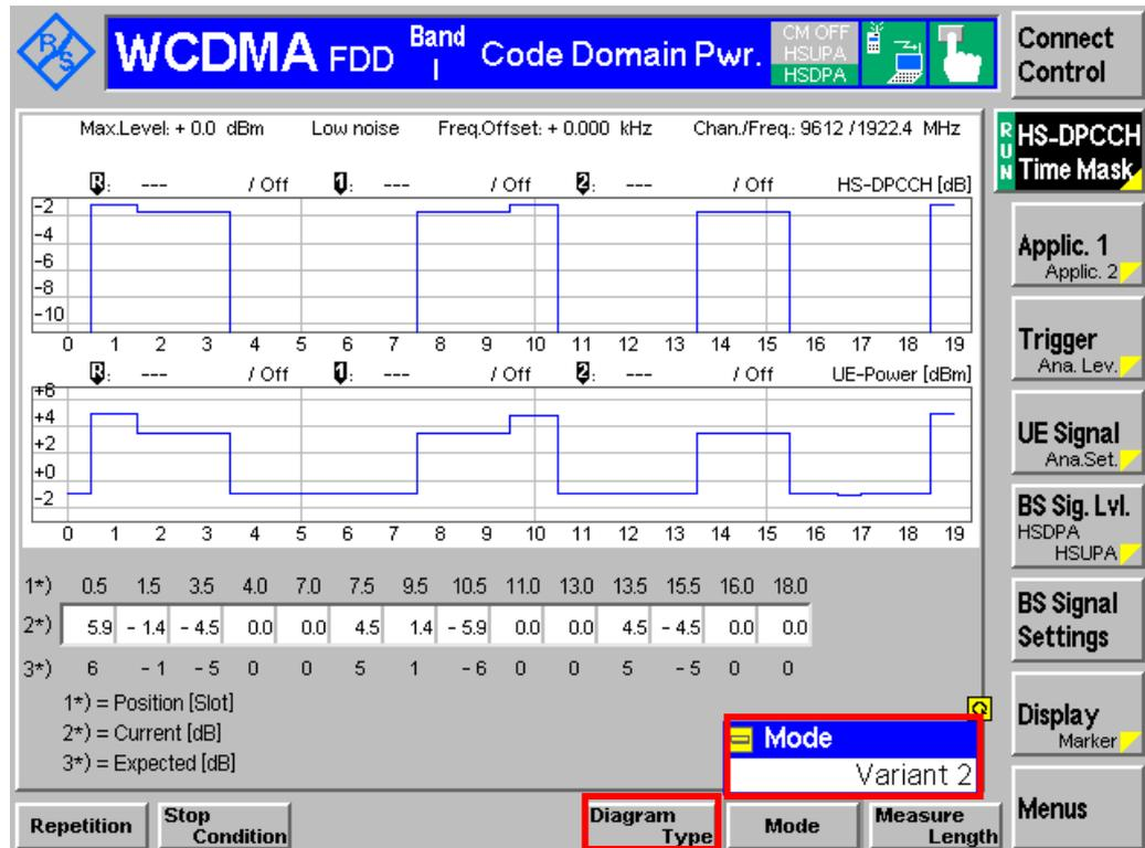
Figure 19: HS-DPCCH power control measurement result
