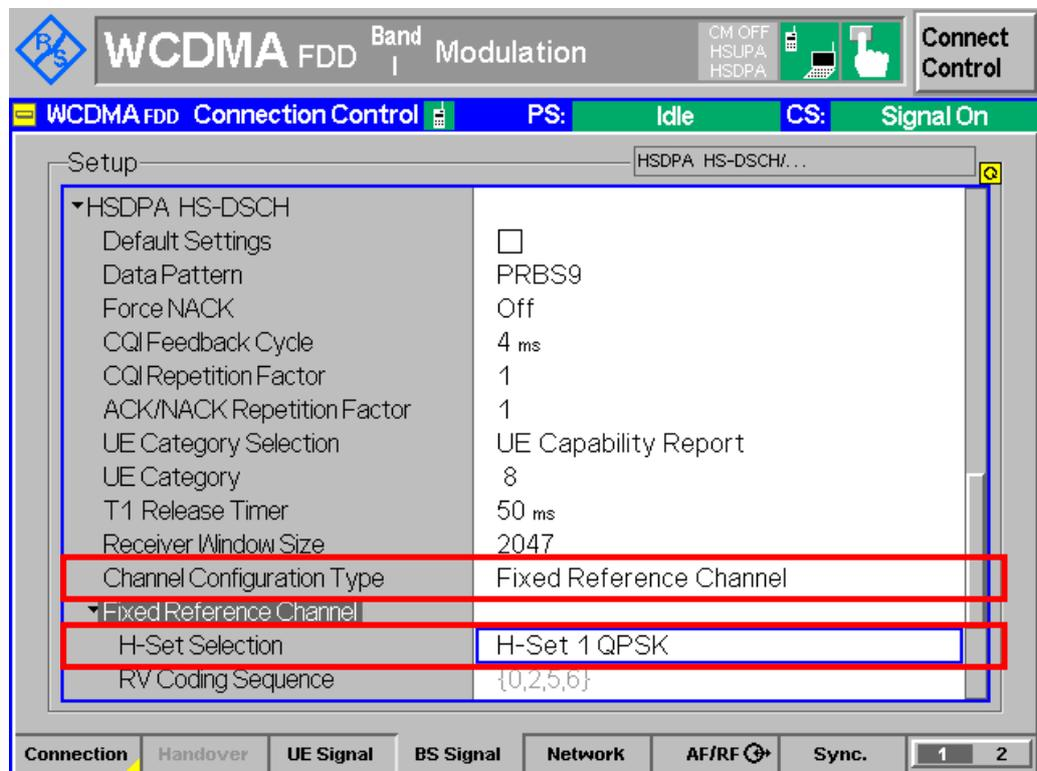
**Figure 5: Fixed Reference Channel configuration**
