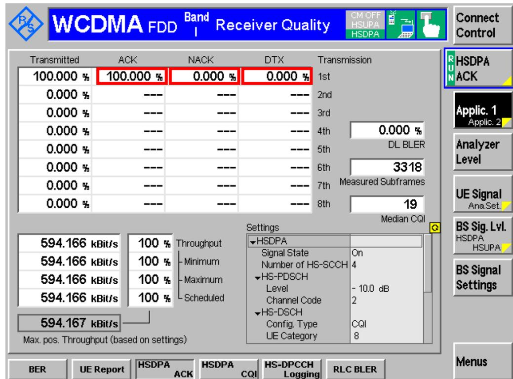
Figure 32: HS-SCCH detection performance – single link performance measurement result
