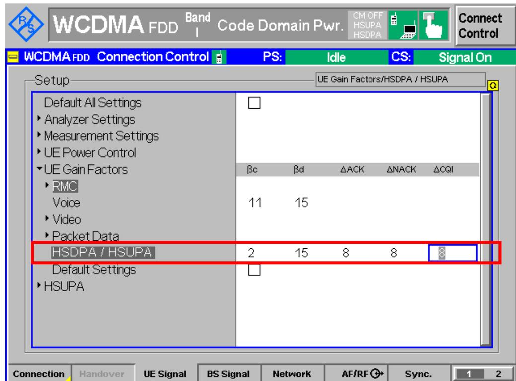
Figure 4:  $\beta$  values for transmitter characteristics tests with HS-DPCCH configuration
