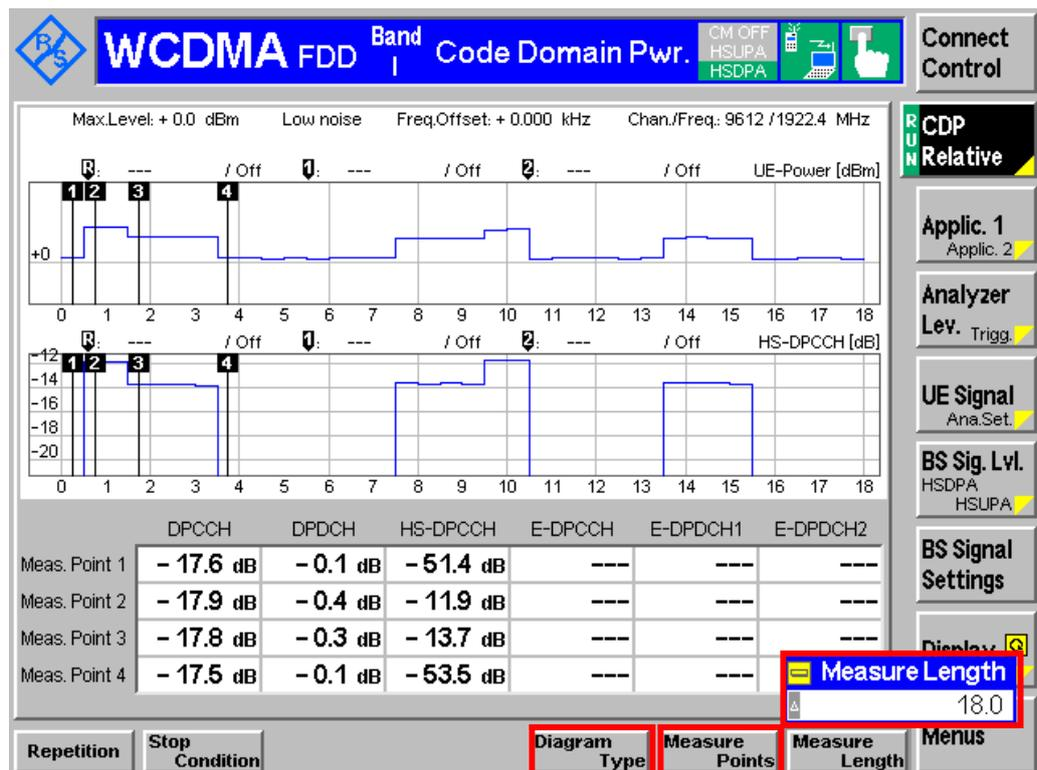
Figure 14(a): UE relative code domain power accuracy measurement result
