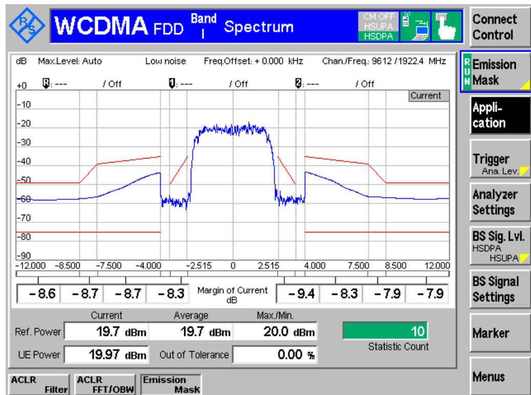
Figure 20: Spectrum emission mask measurement result
