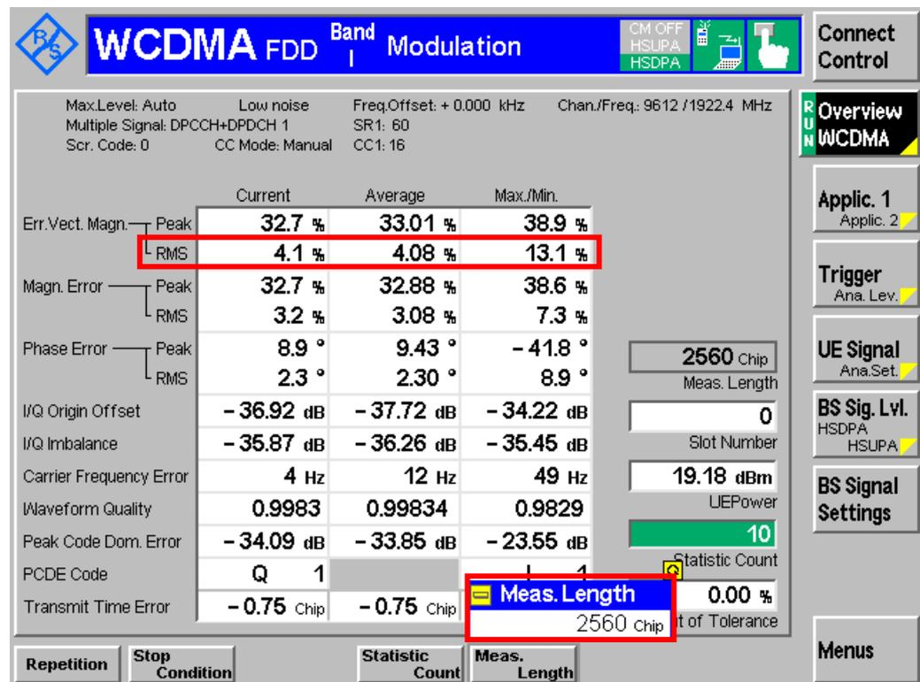
Figure 24: EVM with HS-DPCCH measurement result
