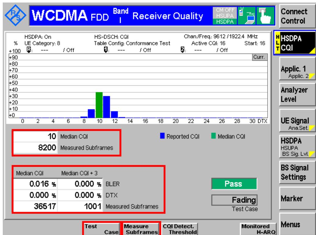
Figure 31: HSDPA CQI (fading propagation conditions) measurement result
