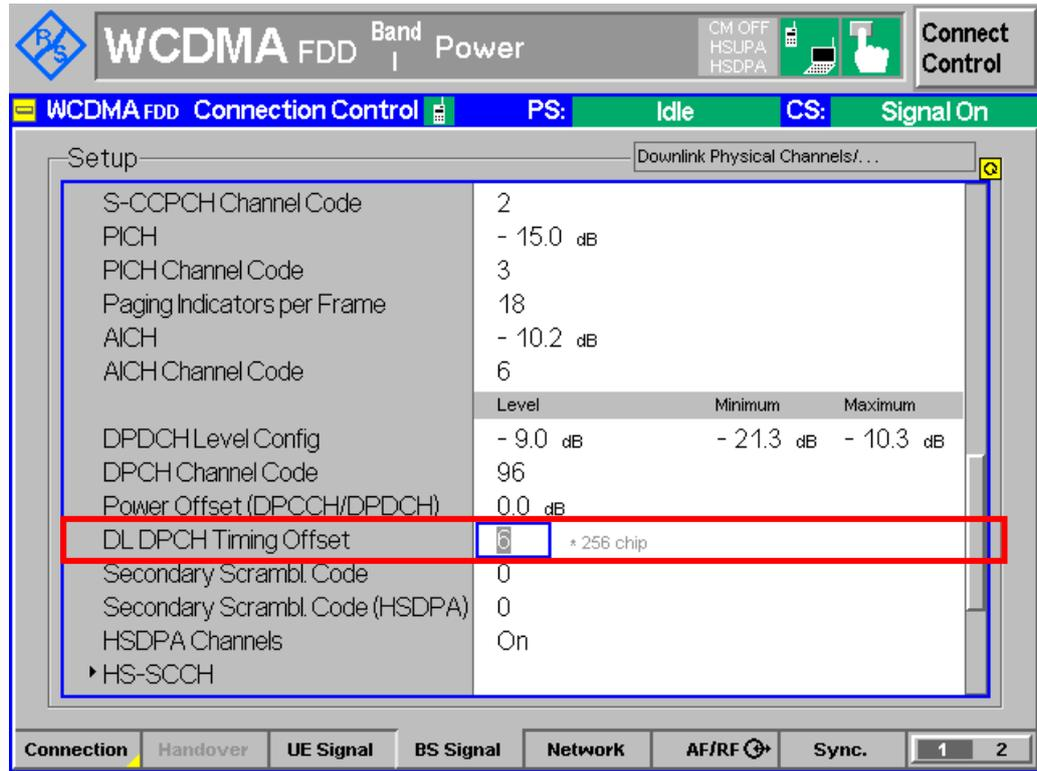
Figure 3: DPCH timing offset configuration
