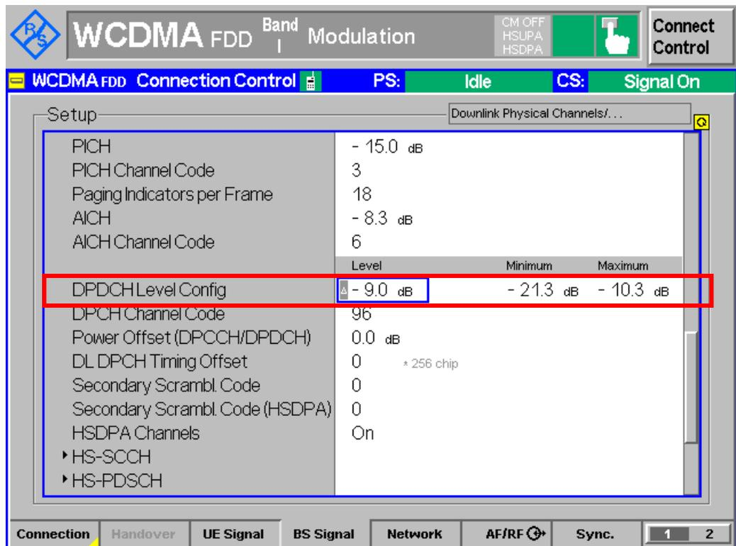
Figure 6(c): Downlink physical channels configuration according to Table 5(a) and Table 5(b)
