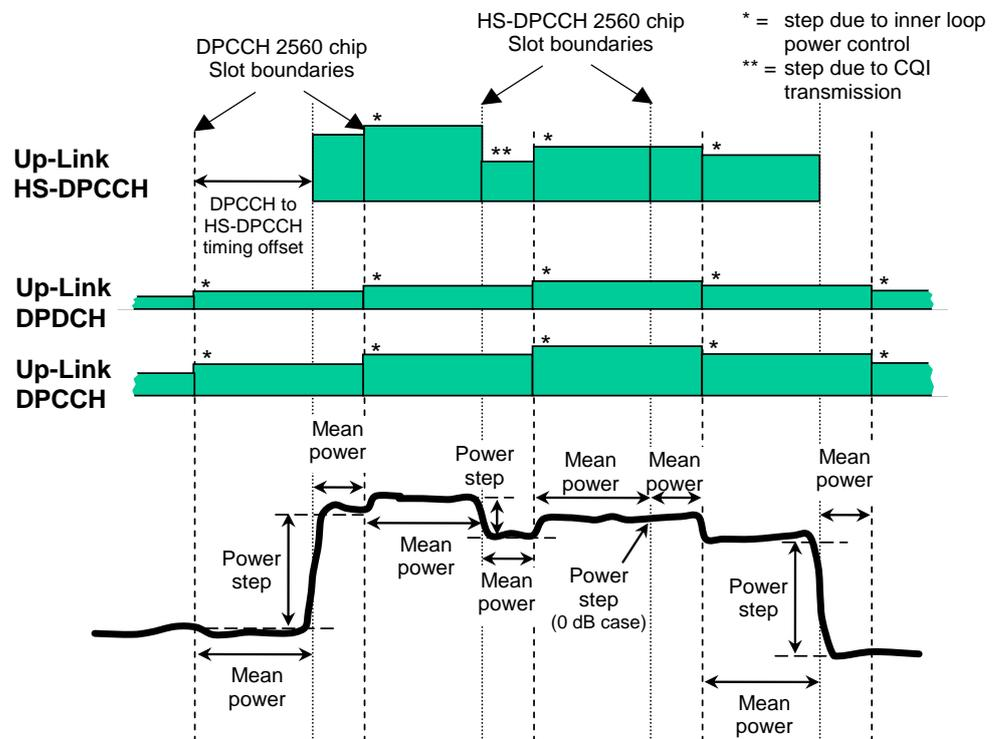
The power step due to HS-DPCCH transmission is the difference between the mean powers transmitted before and after an HS-DPCCH slot boundary. The mean power evaluation period excludes a 25 $\mu$ s period before and after any DPCCH or HS-DPCCH slot boundary.
