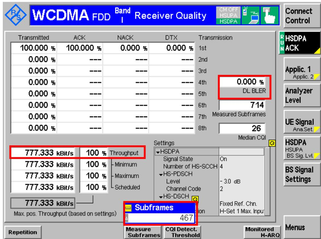
Figure 27: Maximum input level for HS-PDSCH reception (16QAM) measurement result
