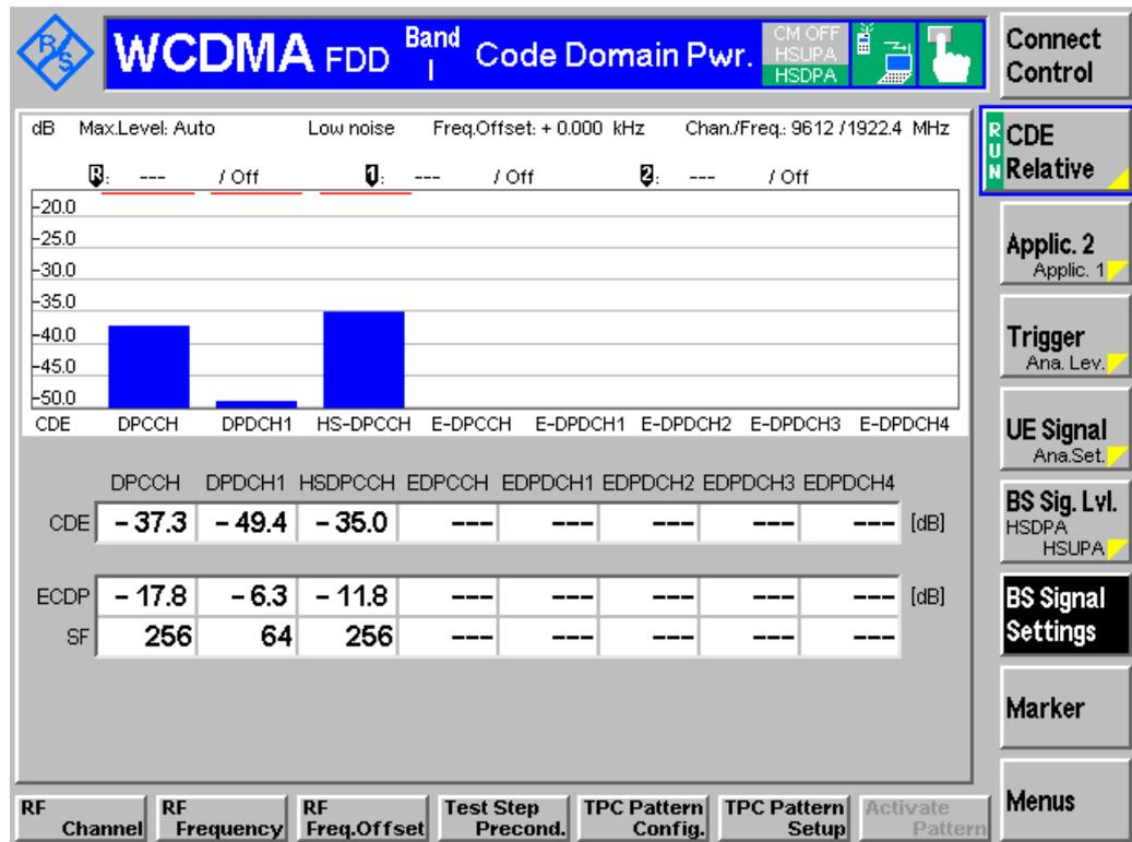
Figure 26: Relative code domain error with HS-DPCCH measurement result
