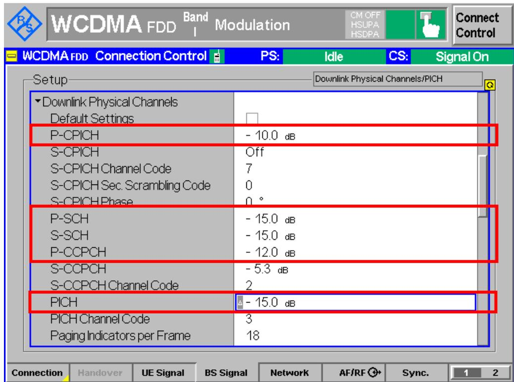
Figure 6(b): Downlink physical channels configuration according to Table 5(a) and Table 5(b)
