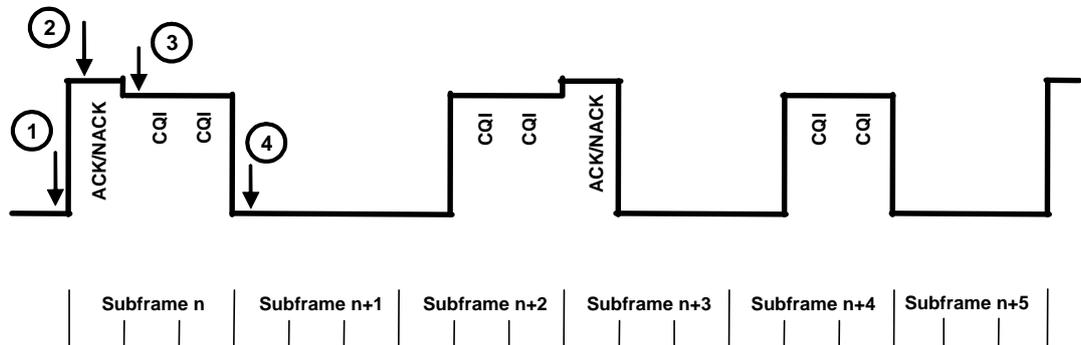
Figure 10: Transmit power profile showing measurement points (Figure 5.2C.1 of TS 34.121 [1])
