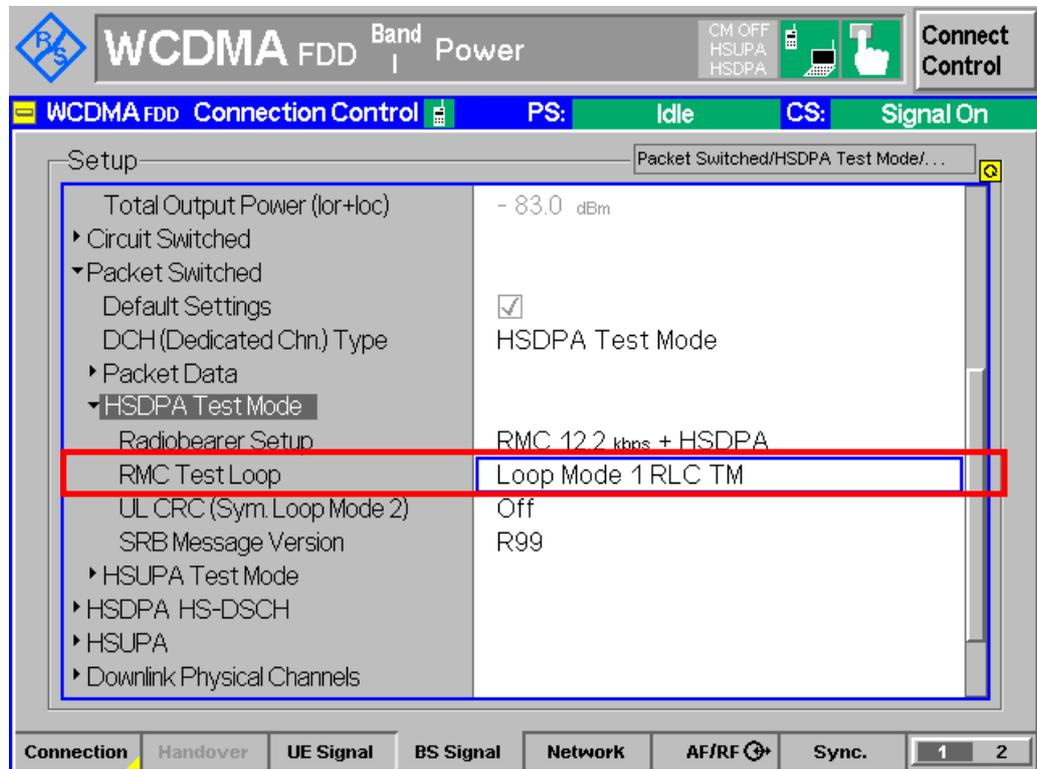
**Figure 11: Loopback test mode 1 configuration**
