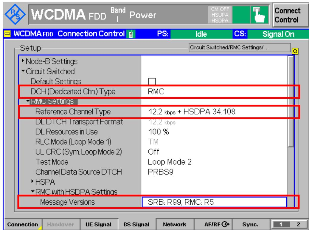
Figure 1(a): RMC 12.2 kbps + HSDPA 34.108 configuration
