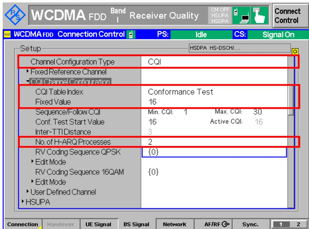
Figure 29: CQI channel configuration
