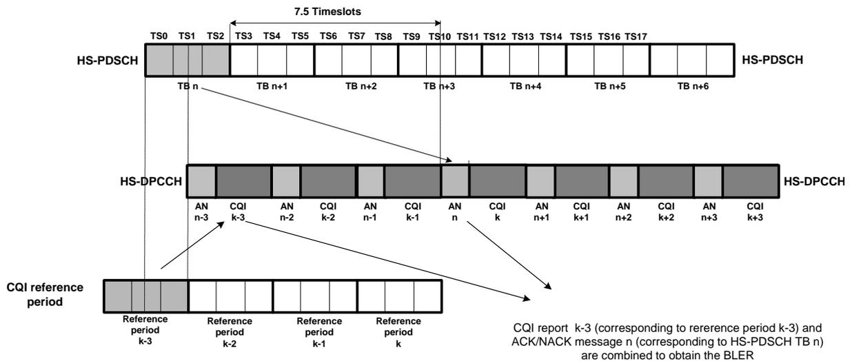
Figure 30: Combination of ACK/NACK message and the CQI report for BLER calculation (Figure 9.3.2.1 of TS 34.121 [1])
