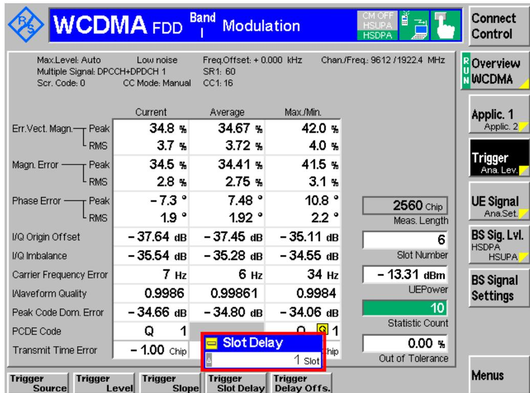
Figure 23(b): Trigger slot delay configuration
