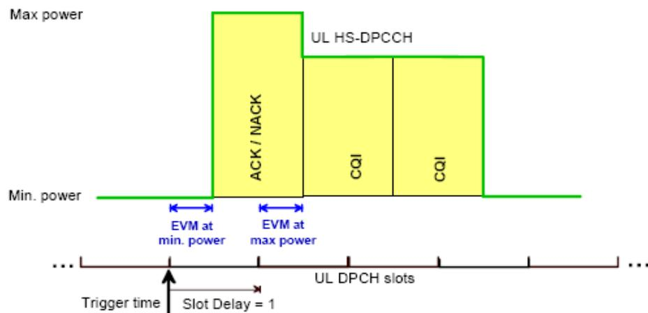
**Figure 23(a): Trigger configuration in R&S<sup>®</sup>CMU200**
