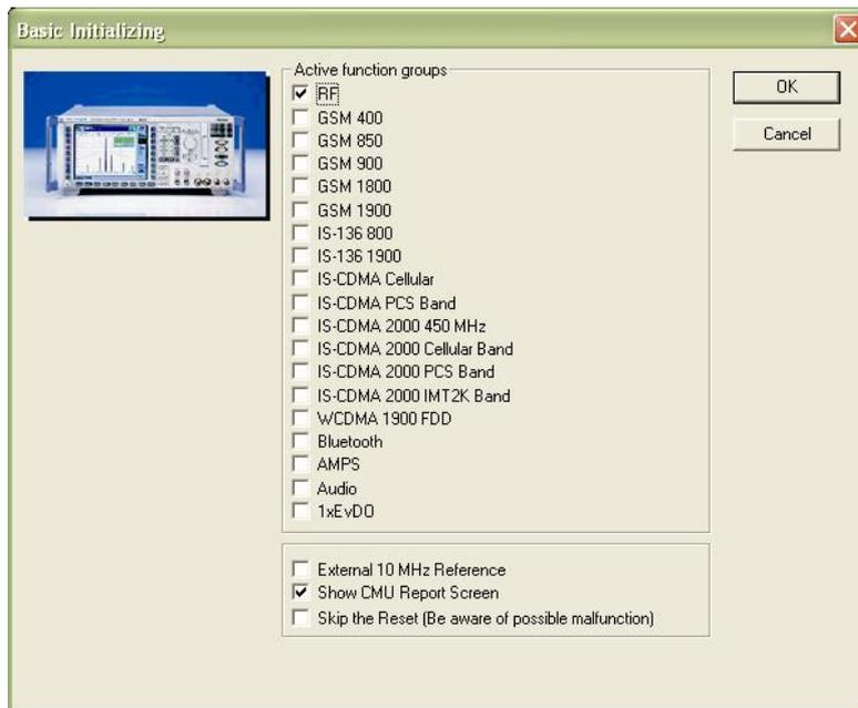
"Basic Initializing" is always at the beginning of a remote-control sequence. In this test item, the available R&S CMU 200 options are queried. In addition, addresses are mapped, i.e. the individual secondary addresses are assigned to the appropriate function groups.
