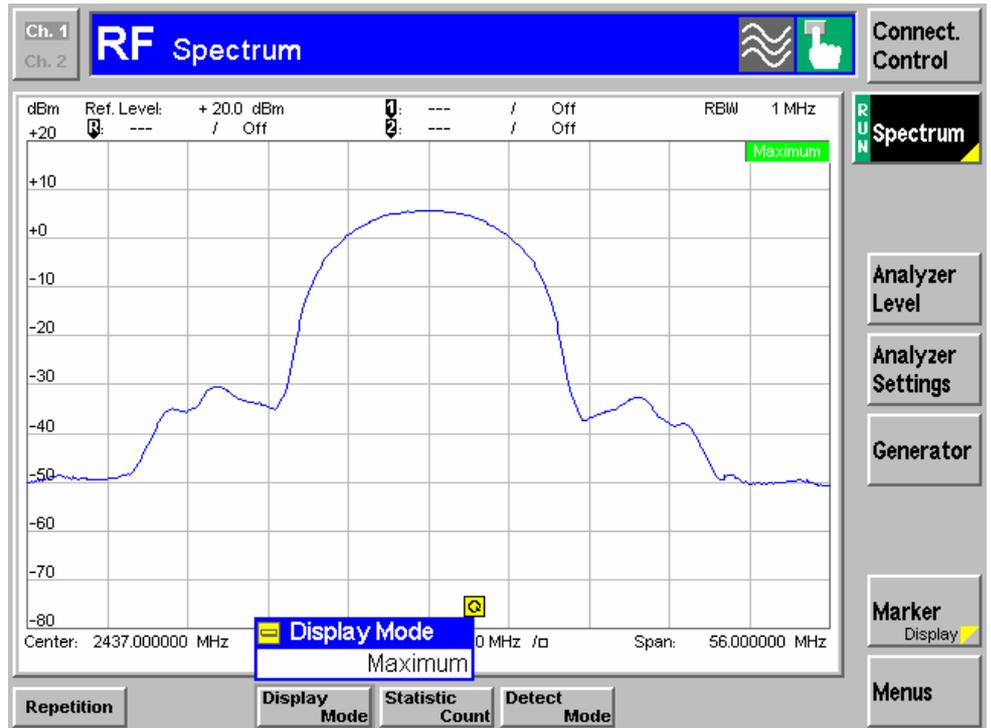
Good results are obtained with an averaging factor of 5, as is shown above. An averaging factor of 2, in contrast, still produces an undesirable number of dips, as shown in the following screenshot:
