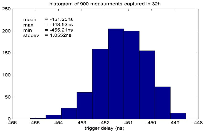
Figure 6: Longterm stability measurement
