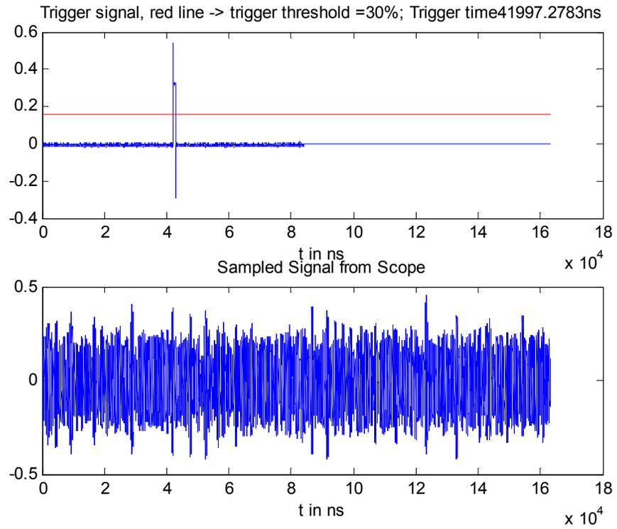
Figure 4: Trigger signal versus sampled CDMA signal
