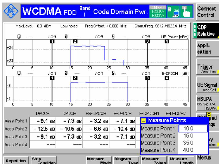
Figure 18: Measure points for relative CDP accuracy measurement.
