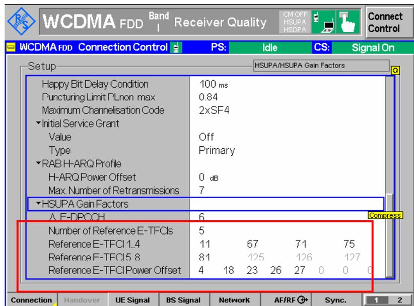
Figure 11: HSUPA gain settings for Tx subtest 1,2,4,5
