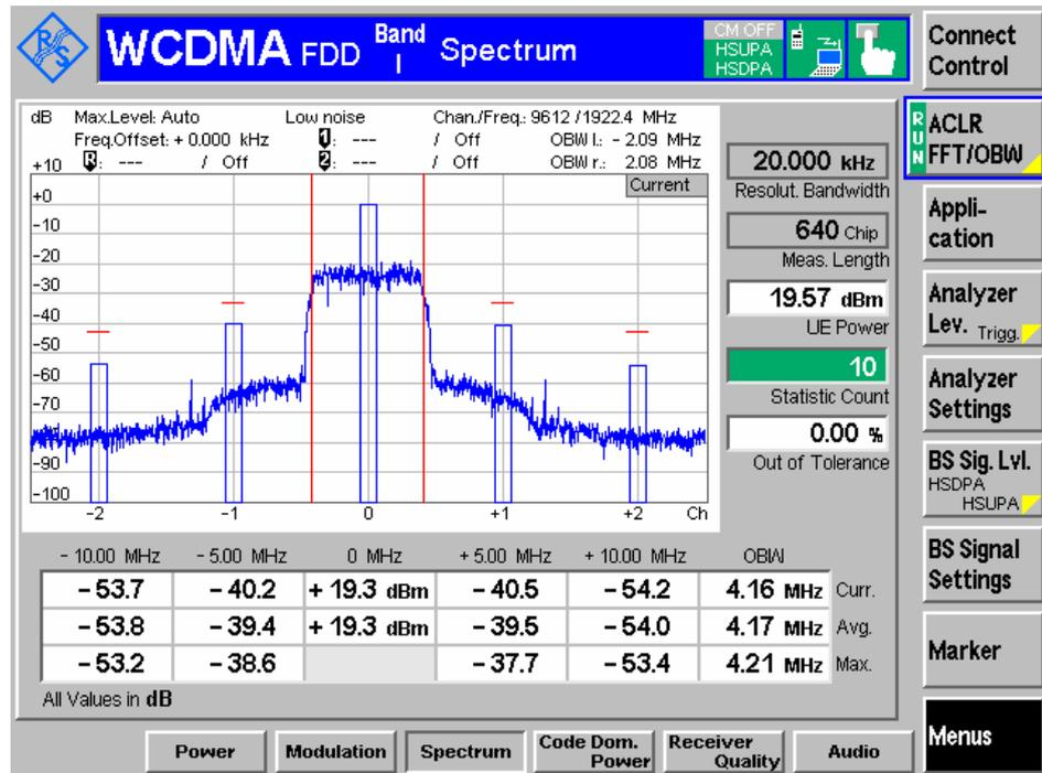
Figure 16: ACLR with E-DCH measurement
