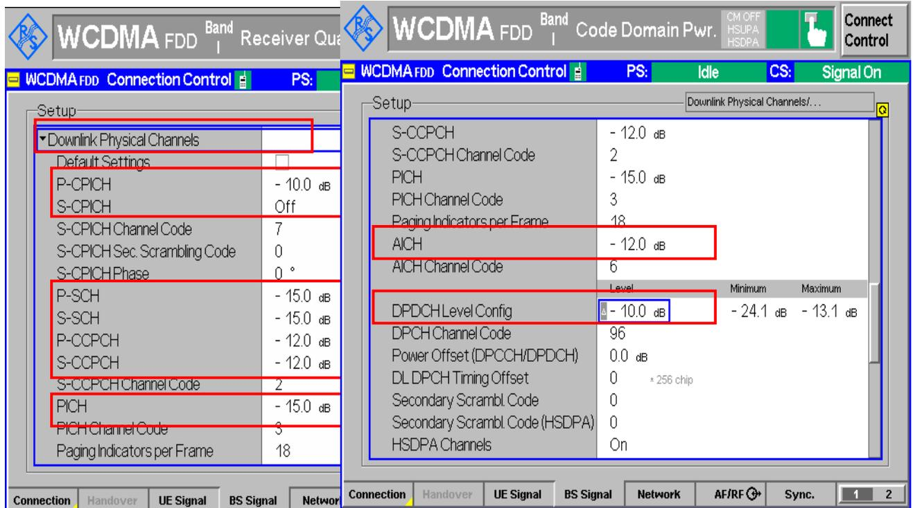
Figure 5: WCDMA downlink channel power level settings
