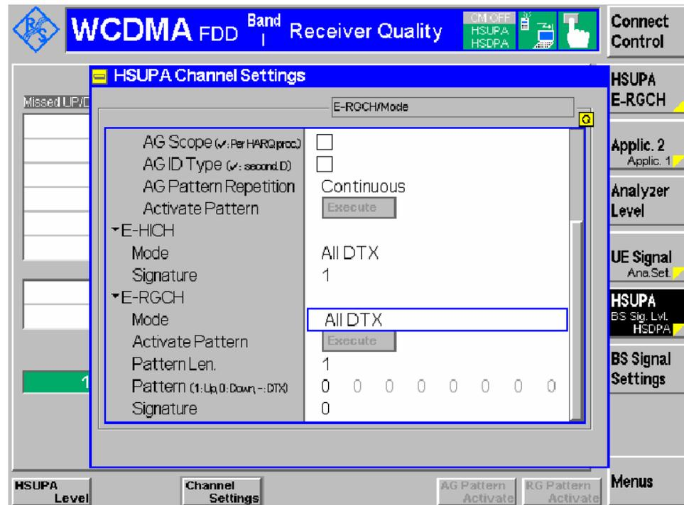
*Figure 37: 'Missed HOLD' test setting for TC 10.3.1.1*
