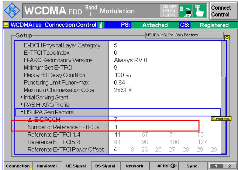
Figure 45: HSUPA Gain Factors setting for TC 10.4.1
