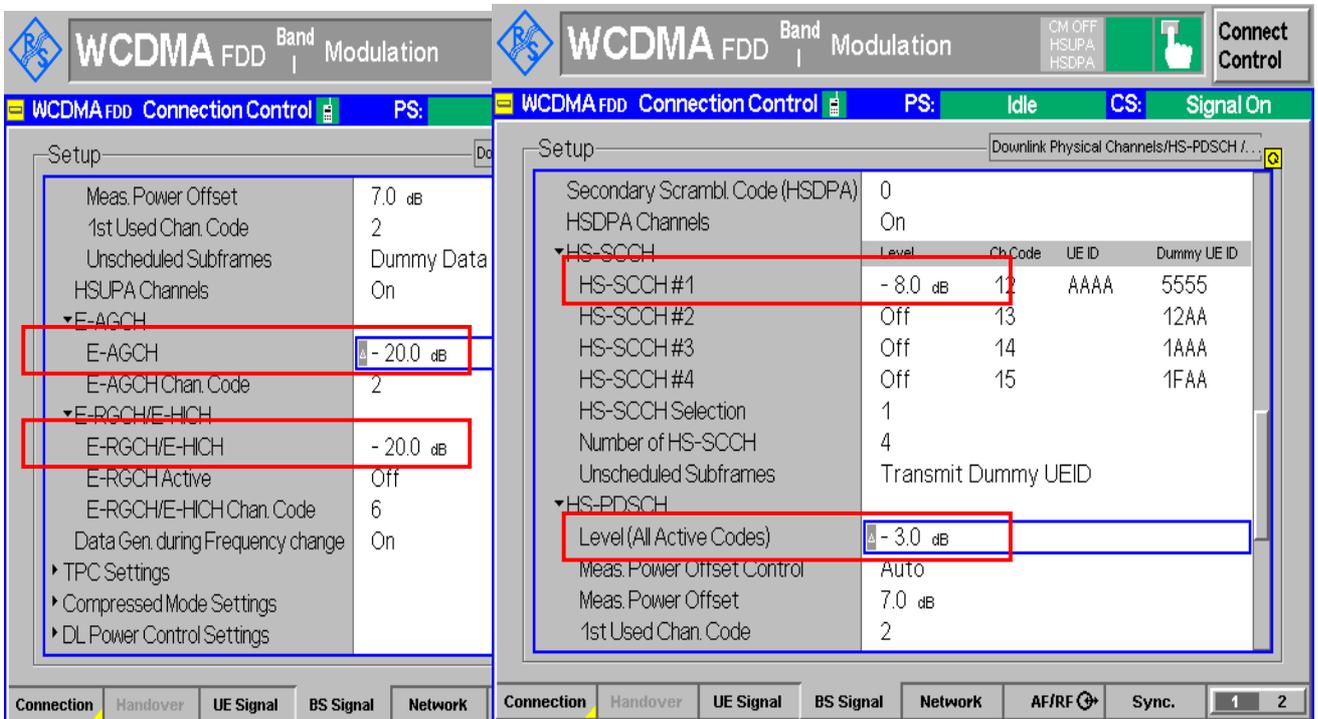
Figure 6: HSUPA power settings for Tx test
