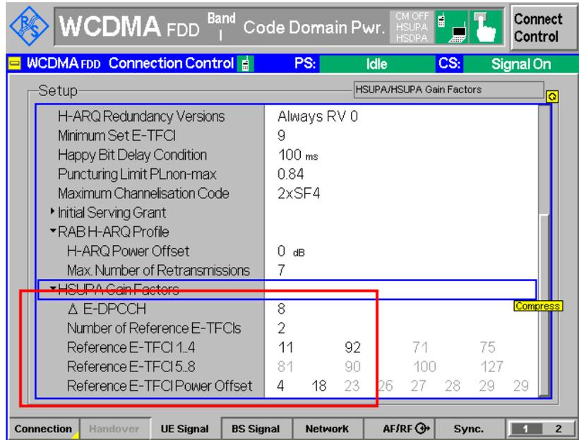
Figure 12: HSUPA gain settings for Tx subtest 3
