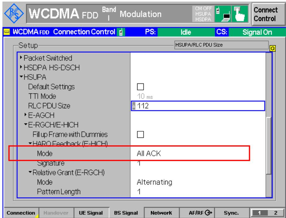
Figure 28: Missed Ack test setting for TC 10.2.1.1
