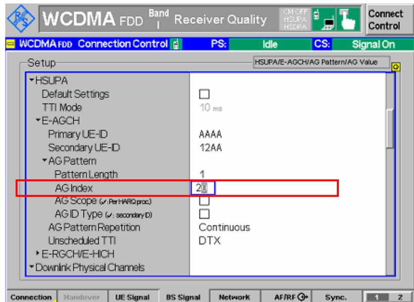
Figure 9: AG Index setting for Tx subtest 1
