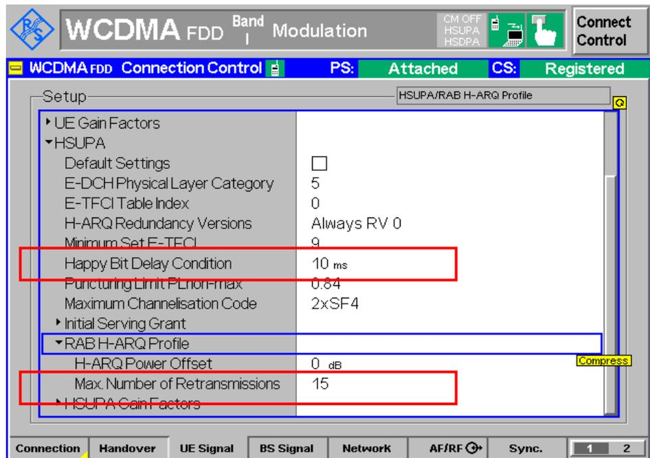
Figure 26: Happy Bit and Retransmissions setting for TC 10.2.1.1
