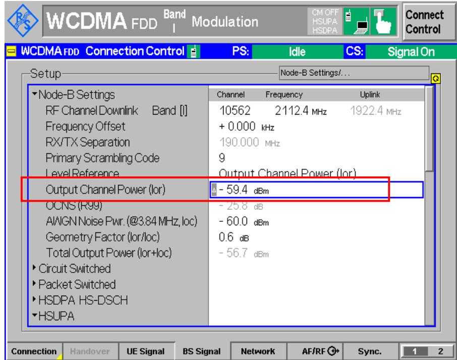
Figure 39: Output Channel Power for TC 10.4.1
