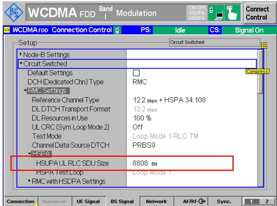
Figure 43: HSUPA UL RLC SDU Size setting for TC10.4.1
