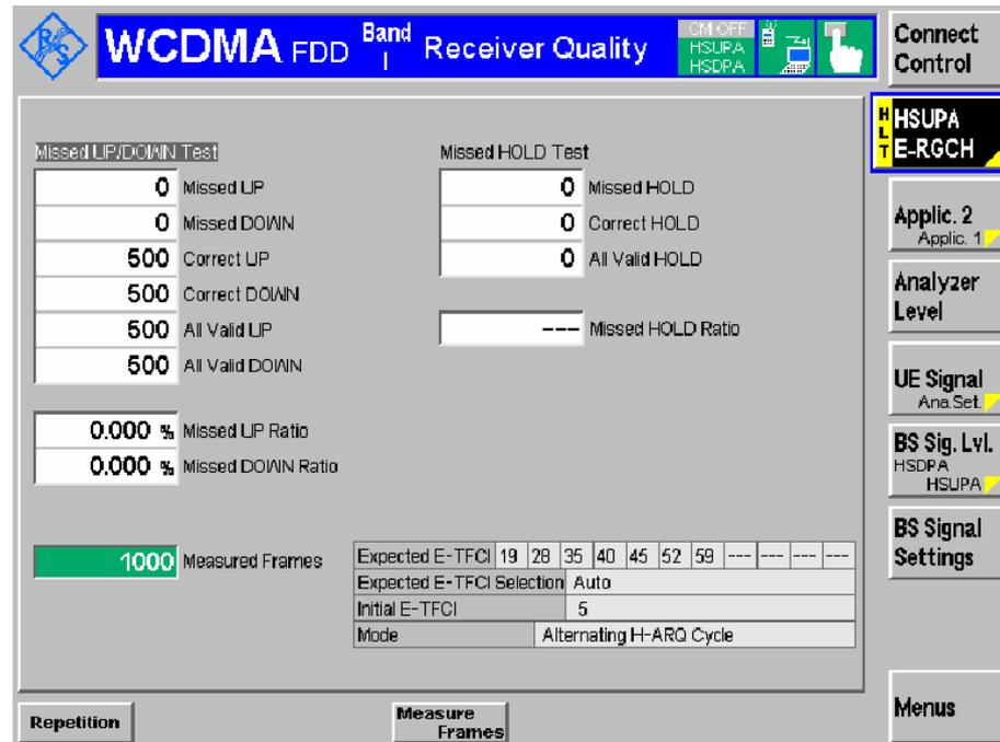
Figure 35: E-RGCH measurement for TC 10.3.1.1
