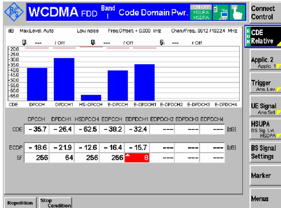
Figure 19: Code Domain Error measurement for TC 5.13B.2
