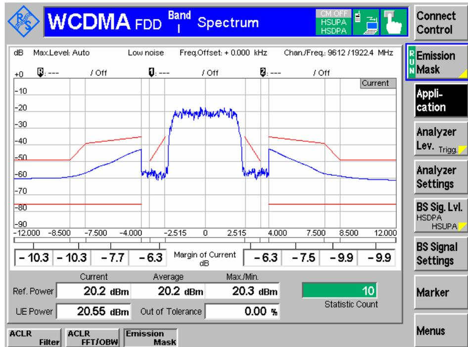
Figure 15: Spectrum emission mask with E-DCH
