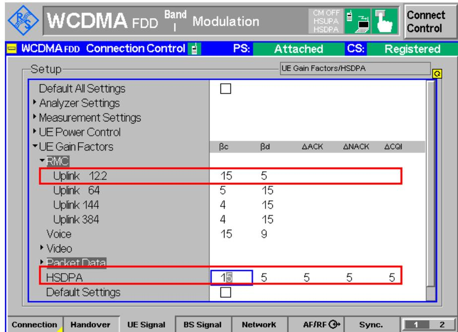
Figure 41: RMC and HSDPA gain setting for TC 10.4.1
