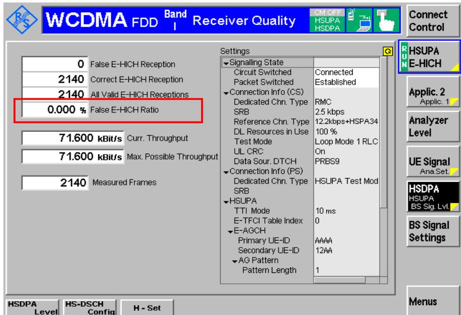
Figure 29: Missed Ack test result for TC 10.2.1.1
