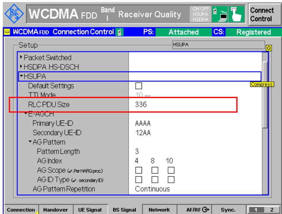
Figure 44: HSUPA UL RLC PDU Size setting for TC 10.4.1
