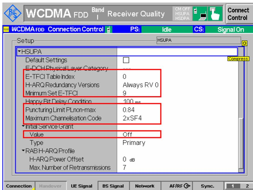
Figure 8: HSUPA signaling setting for Tx test
