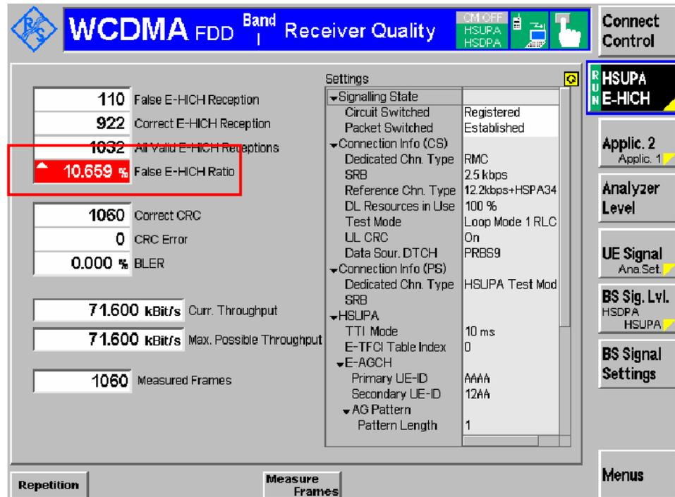
Figure 31: False Ack test result for TC 10.2.1.1
