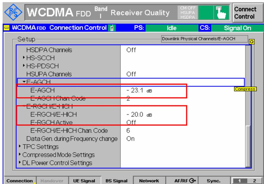
Figure 40: HSUPA channel power level setting for TC 10.4.1
