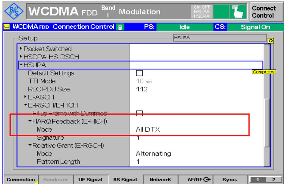
*Figure 30: False Ack test setting for TC 10.2.1.1*
