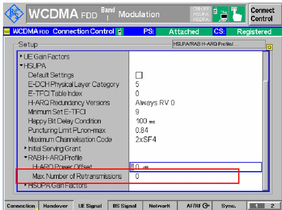
Figure 42: Maximum number of retransmissions setting for TC 10.4.1
