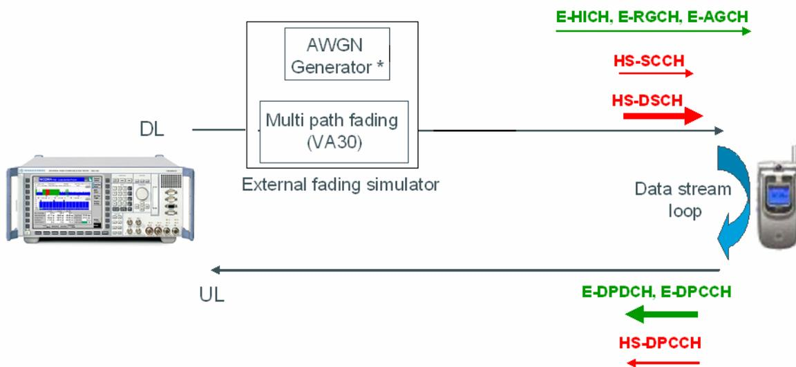
*Figure 20: Px test setup*
