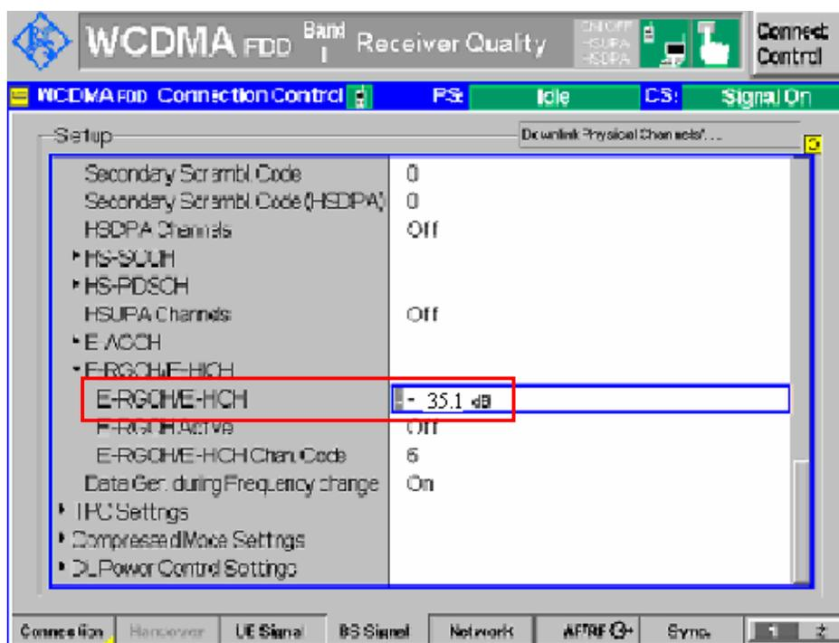
**Figure 24: E-RGCH/E-HICH power level setting for TC 10.2.1.1**
