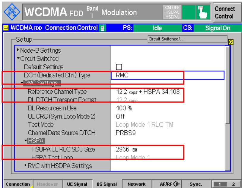
Figure 2: RMC Setting for HSUPA test
