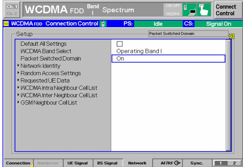
Figure 1: Activate packet switched domain
