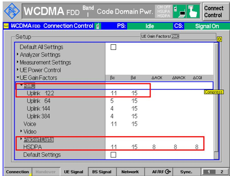
Figure 10: RMC and HSDPA channel gain settings for Tx subtest 1
