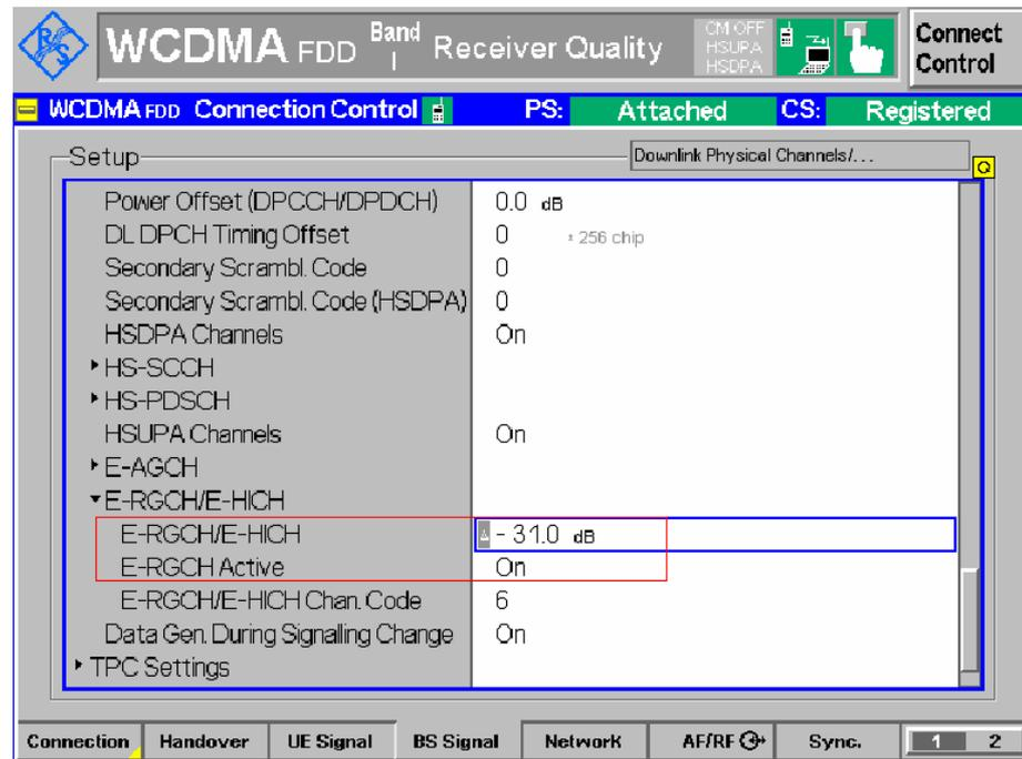
Figure 32: Activate E-RGCH channel and E-RGCH power setting
