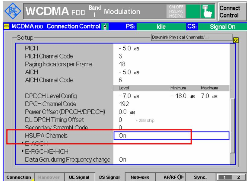
Figure 3: Activate HSDPA and HSUPA channels
