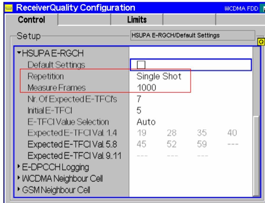
Figure 36: Configure the single shot test for TC 10.3.1.1
