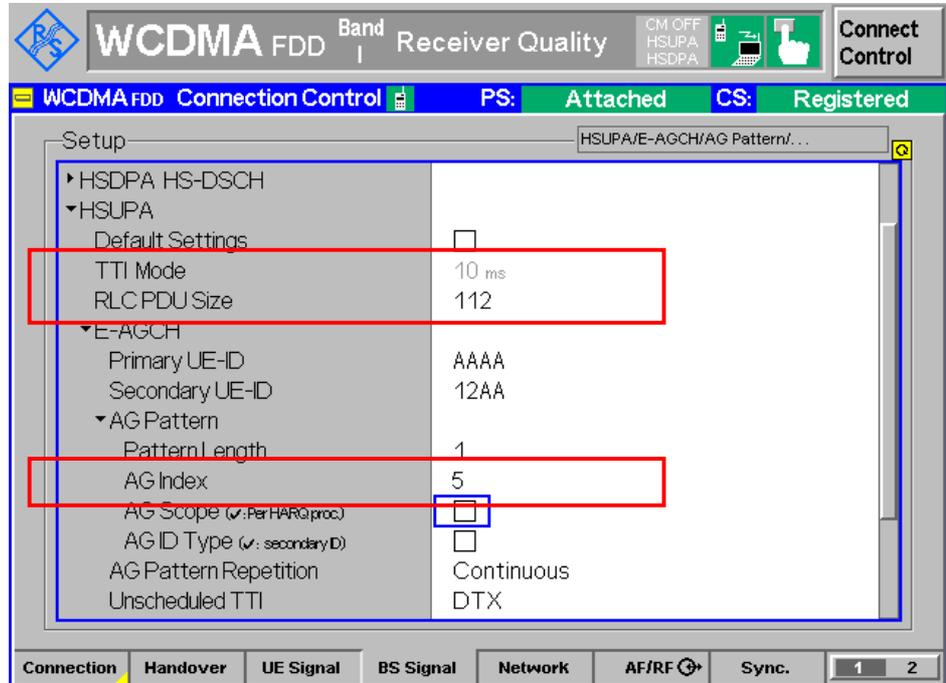
Figure 25: AG Index and RLC PDU Size setting for TC 10.2.1.1
