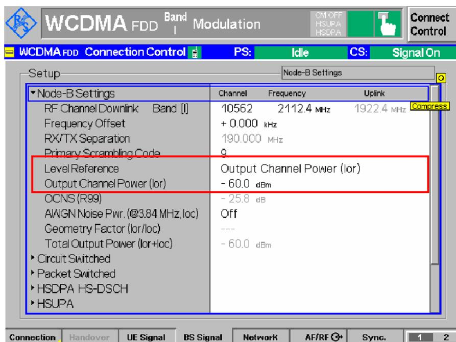
Figure 21: Output channel power for Px test
