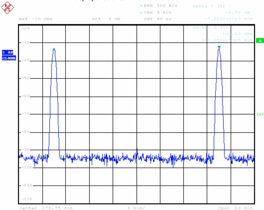
*Figure 16 The level difference between both carriers must be within a certain margin to obtain accurate IMD measurements*
