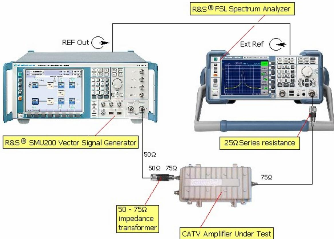
Figure 13 Test set-up for IMD test
