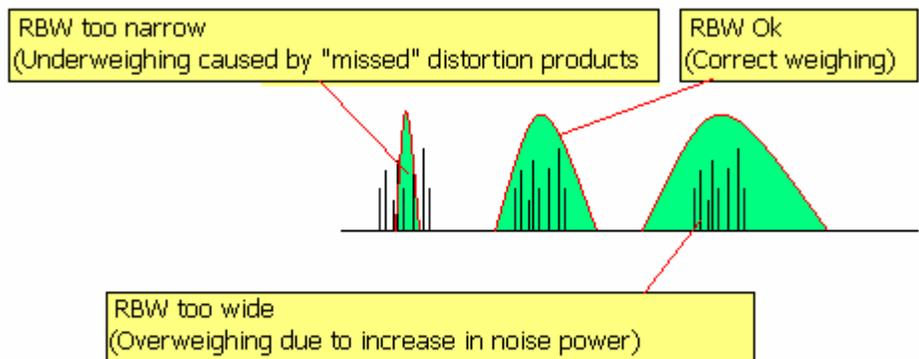
Figure 9 Effect of the *RBW* on the result of CSO & CTB measurements
