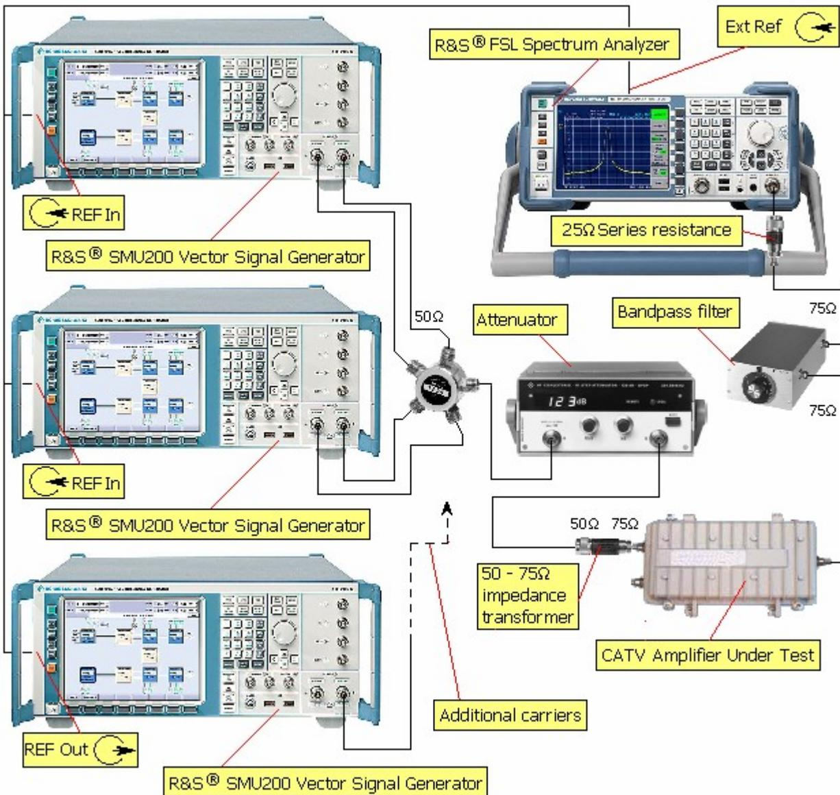
Figure 19 Test set-up for CTB test
