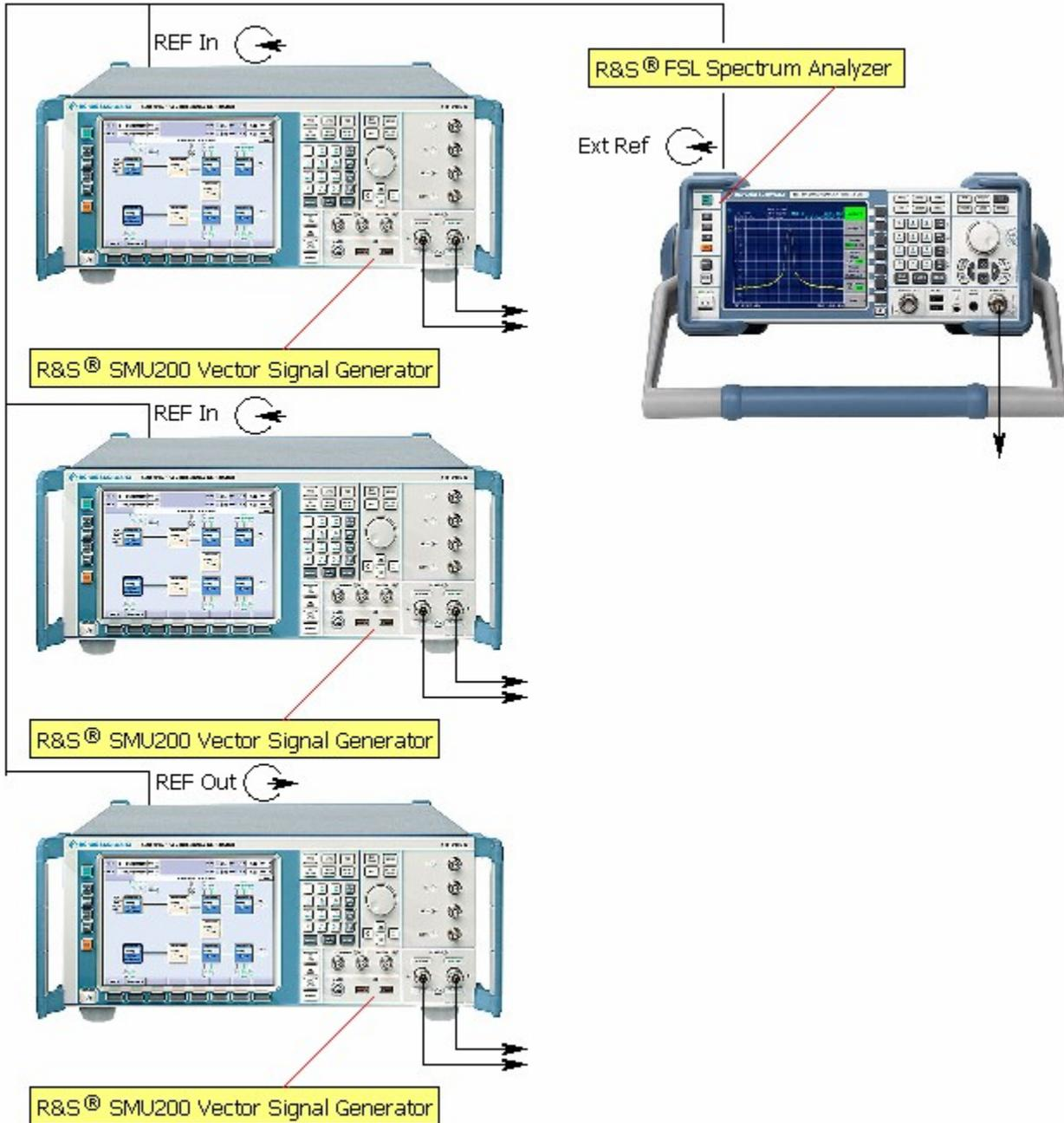
Figure 12 Set-up for improved composite intermodulation distortion measurements
