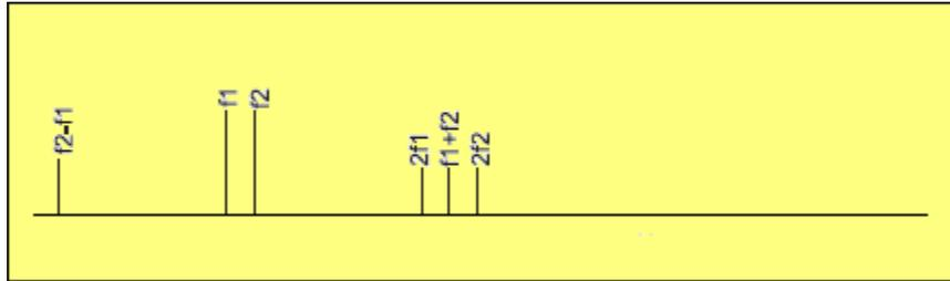
*Figure 2 “Two-tone” 2<sup>nd</sup> order intermodulation products for a device with 1<sup>st</sup> and 2<sup>nd</sup> order terms in its transfer function*
