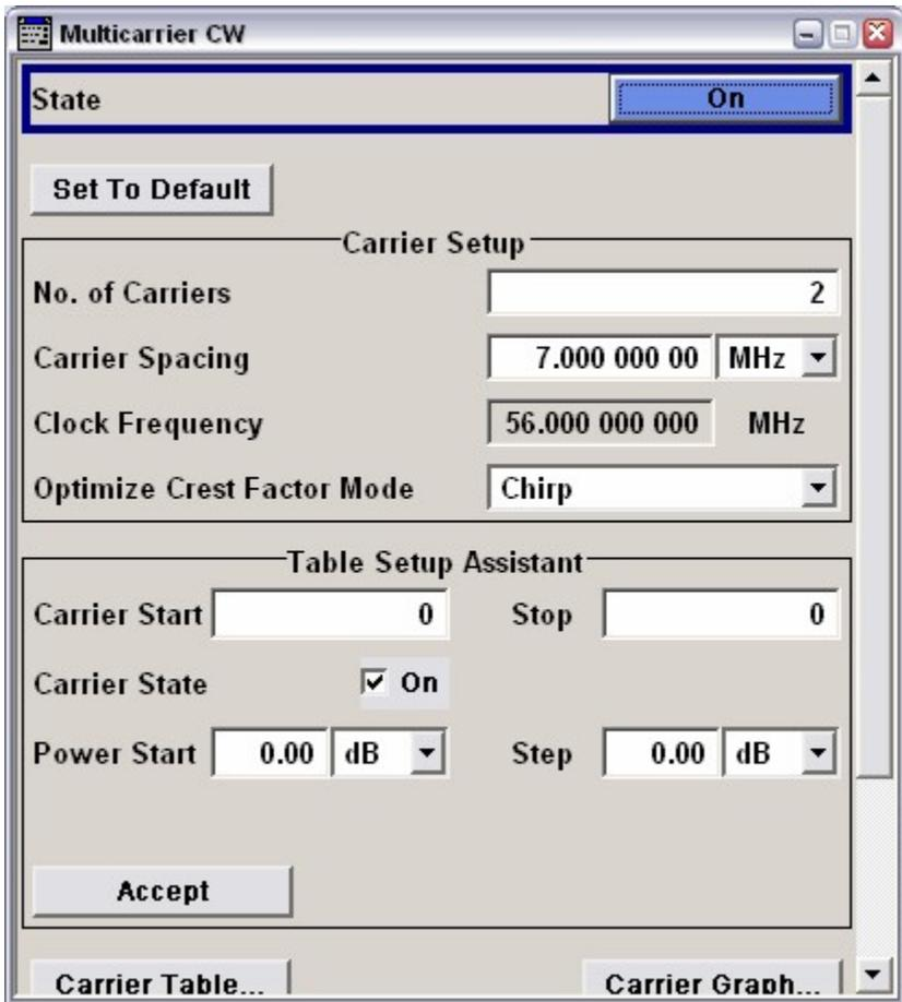
Figure 15 Multicarrier settings window
