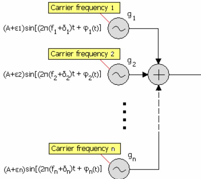
*Figure 8 Multiple carrier signal generated with discrete oscillators*
