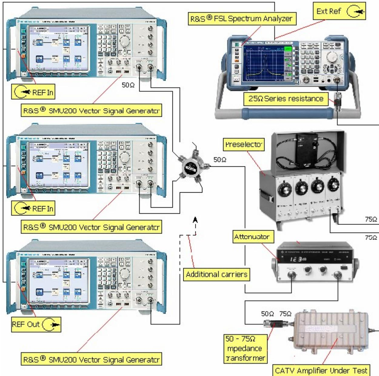
Figure 26 Test set-up for XMOD test
