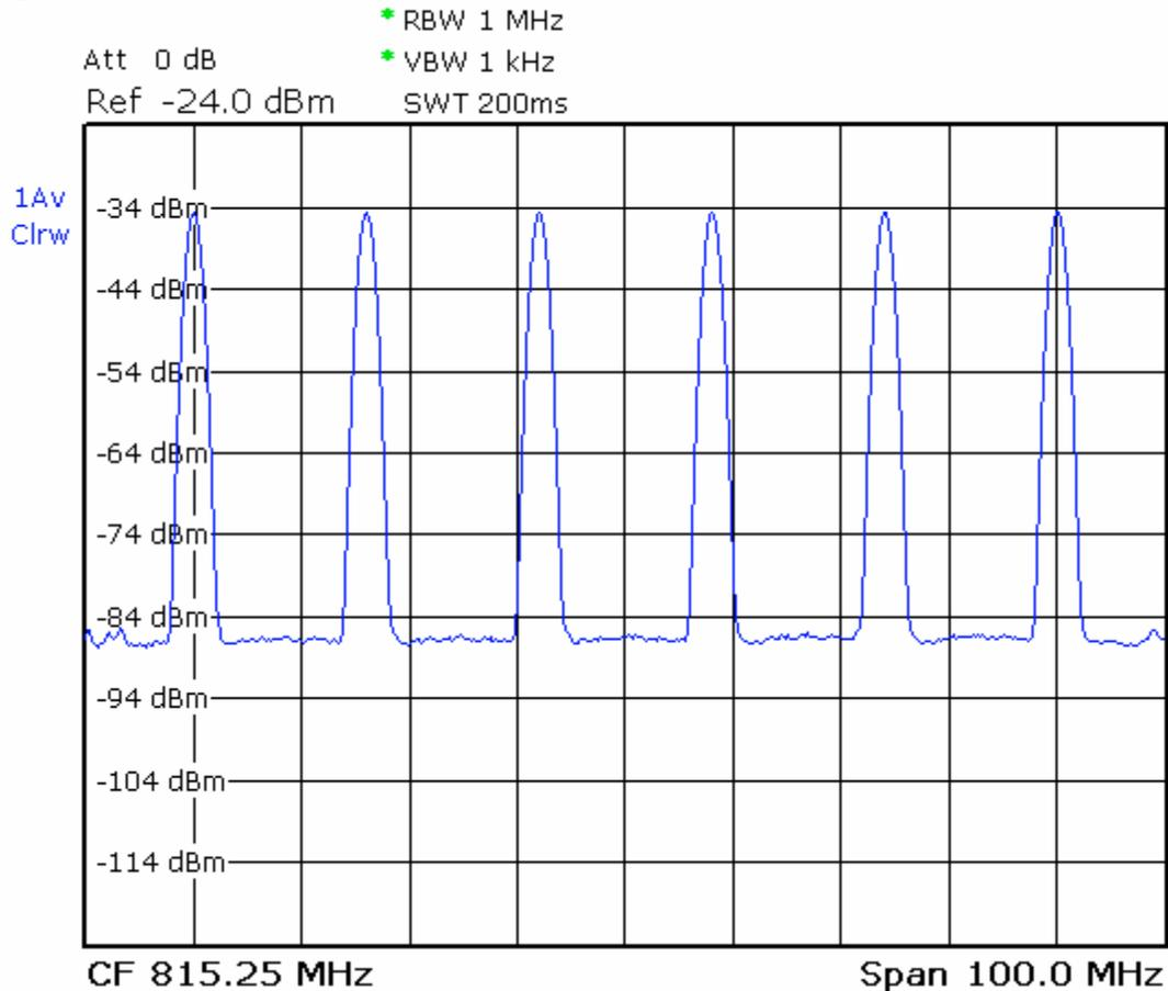
Figure 24 CATV multi-carrier signal with 6 carriers
