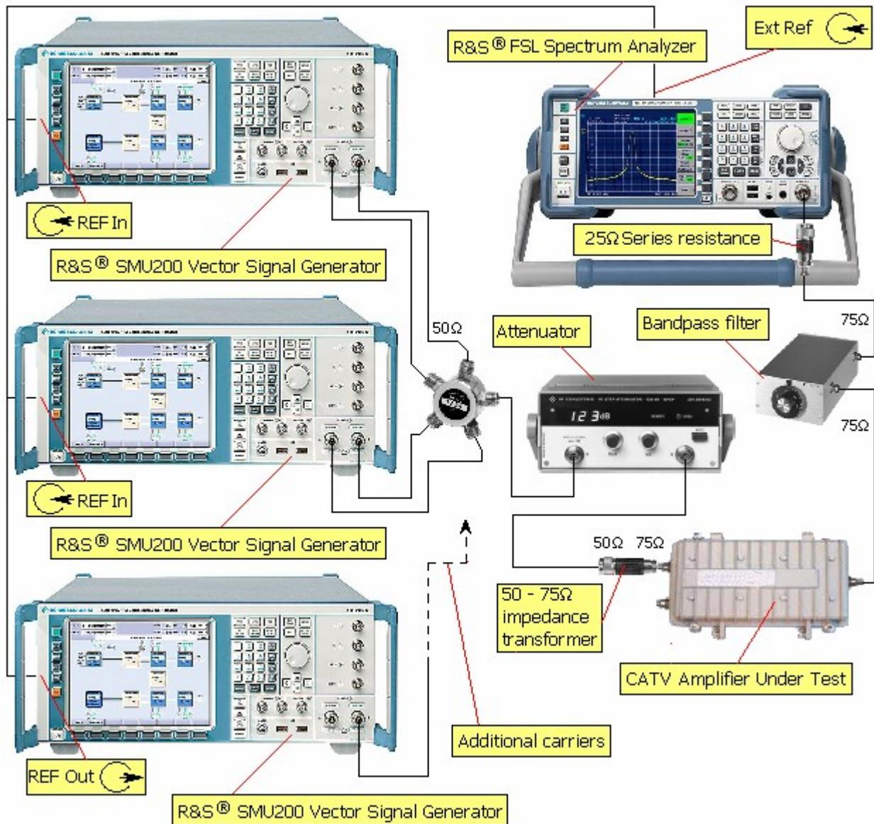
Figure 25 Test set-up for CBT measurement
