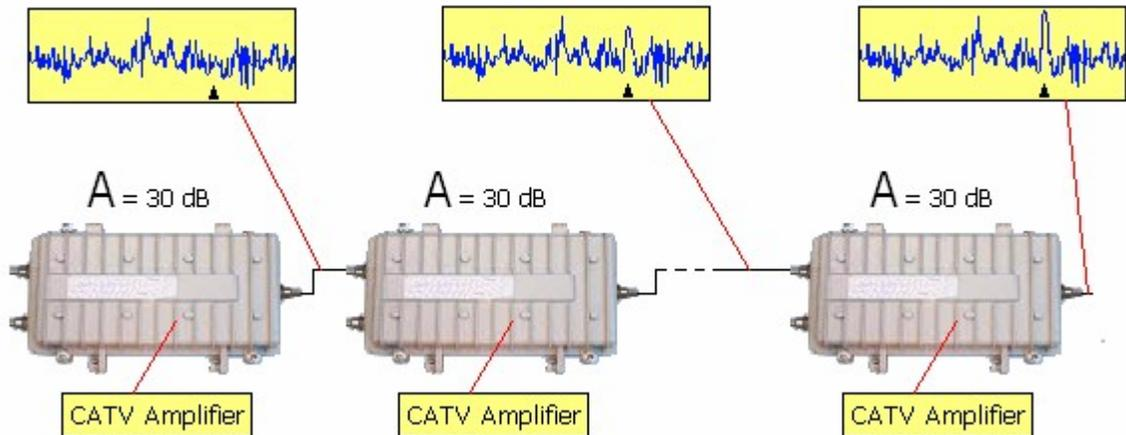
*Figure 10 Cascading effect of amplifiers*
