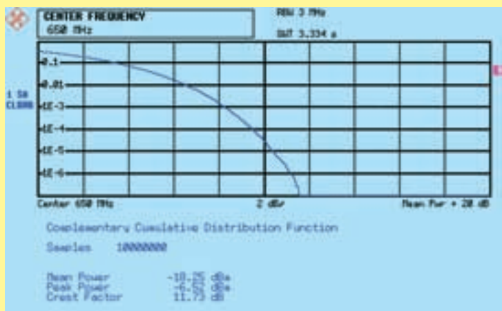
FIG 4 CCDF measurement with the Spectrum Analyzer FSP (method 2). Same signal as in FIG 3; the crest factor (11.73 dB) is 3 dB lower than in the measurement according to method 1 (14.7 dB, FIG 3).
